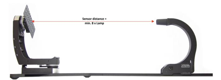
For example, for a lamp with a 20 cm diagonal illuminating surface (the photometrical center being in the middle of the diffuse disc), the distance from center of rotation of the gonio to the sensor should be at least 160cm (20cm x 8). See more in "Guidelines - building a lighting laboratory".
