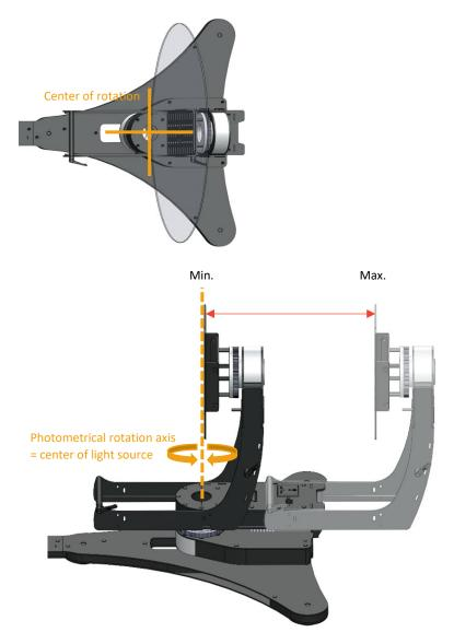
The tower can be adjusted from 0 cm to a max lamp depth of 35 cm.
