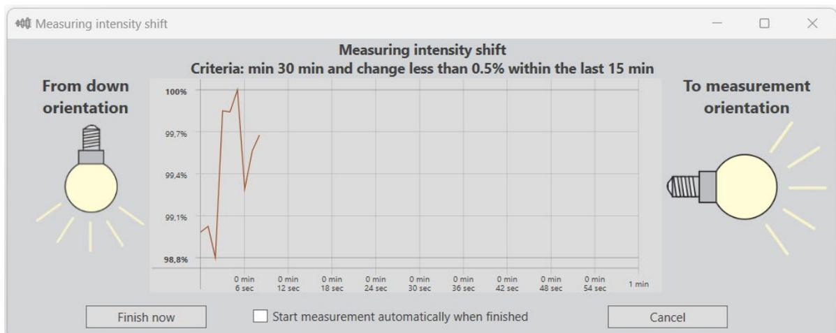
The operator ticks the box “Start measurement automatically” to continue with a normal measurement cycle afterwards (a window opens where you can choose the appropriate qty of measurement planes).
