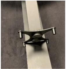
3. The complete LabDisc can now be placed freely on the rail. The correct distance from the LabDisc to the sensor is approximately 50 cm.
