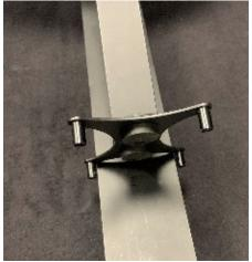
3. The complete LabDisc can now be placed freely on the rail. The correct distance from the LabDisc to the sensor is approximately 40 cm. Check that the distance to the front of the sensor head does not exceed 50 cm. If the distance is too long, the sensor may not "see" the whole light source. If the distance is too short, the disc will not be as effective in reducing straylight from the back wall behind the gonio.
