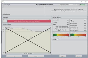
This cross will also be shown on the LabFlicker device and a new measurement will be required. Simply press the 'Start/Pause' button again. If it is not possible to do a measurement within the 'OK' range of the LabFLicker and the cross is shown both in the display and on top of the result (in Light Inspector), the result can still be saved, but the accuracy of this measurement cannot be guaranteed.
