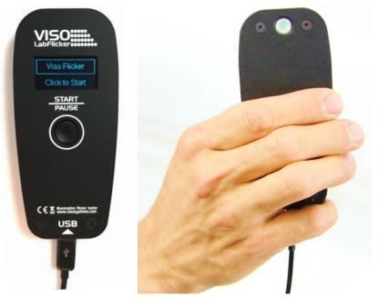
To make a measurement, press the Start/Pause button and move the LabFlicker towards the lamp you want to measure with the sensor facing the lamp.
