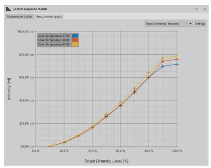
In this view you can see graphical representations of the control sequence data. The default graph shows the measured intensity versus the target dimming level.
