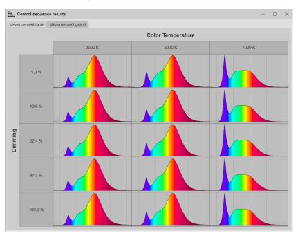
This window displays the number of control steps that were performed as a matrix (2 dimensional or single). In this view, you will just see a small spectrum image that represents each control step.
