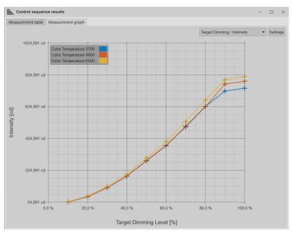
In this view you can see graphical representations of the control sequence data. The default graph shows the measured intensity versus the target dimming level.
