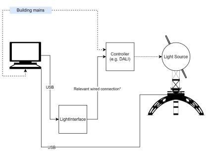
Or use as powered USB hub as intermediate (1 USB cable to measurement PC):
