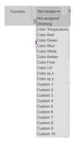
Custom channels can be used to set e.g. tilt or pan of your dmx lamp, to ensure correct settings for every measurement. When assigned, add this parameter to the "main measurement parameters" in the control sequence, and type in the DMX value directly (0-255 or 0-65535).
