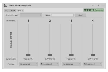
There are four 0-10 V channels to work with. Functions are assigned like with DMX.
