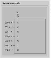
In this area, you can see the steps that will be measured graphically. The matrix illustrates your sequence – choice of parameter setpoints and combinations. Each 'x' represents a measurement.
