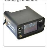
See the flickering light directly with the built-in light source (1100 lm, 3000 K) or turn it off
