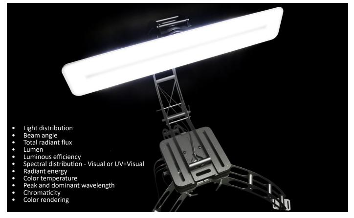
The 2-axis goniometer enables full 3D light measurements
