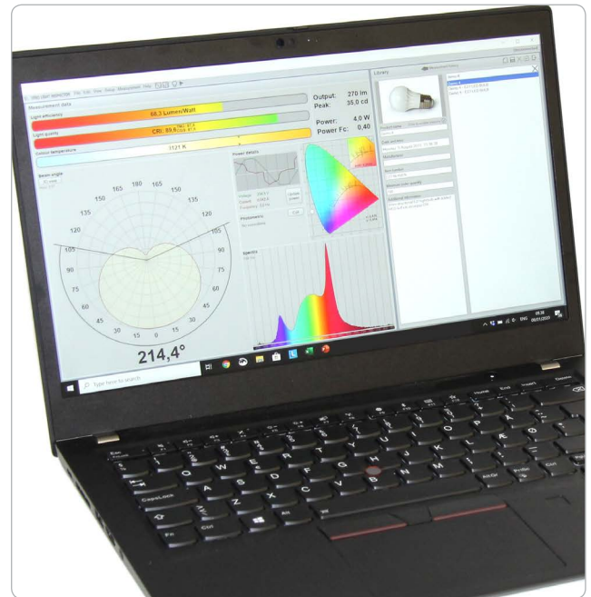
The Viso Light Inspector software is included. The software controls the fully automatic measuring process, all settings and outputs and your measurement library. User-friendly graphics and plenty of output options at your fingertip.
