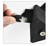
The laser automatically turnes off/on during measurements via Viso Light Inspector software
