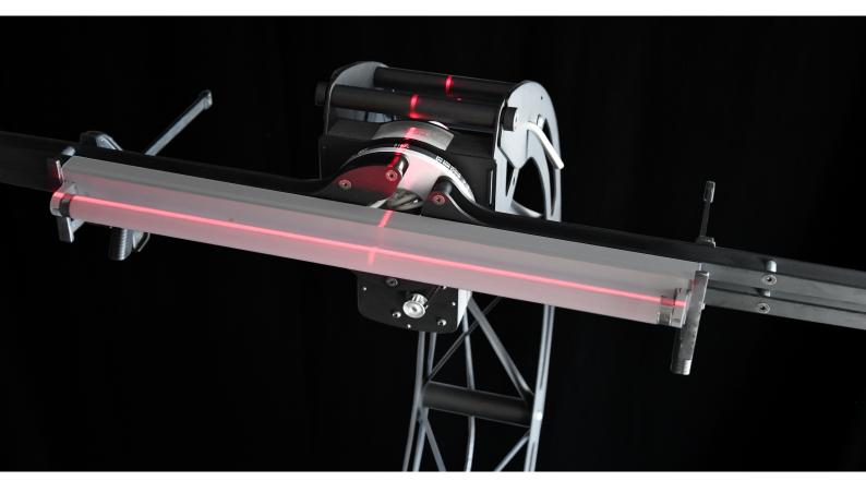
The laser lens can be rotated to be aligned. Horizontal levelling with three screws
