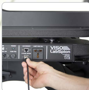
The LabTemp connects to the mainboard with a single Ethernet cable
