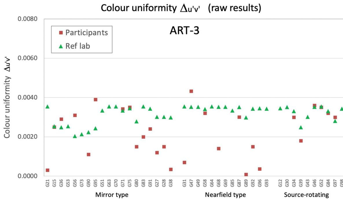
Figure 7-146. Raw results of colour uniformity measured by the participants and the reference lab grouped for each instrument type
