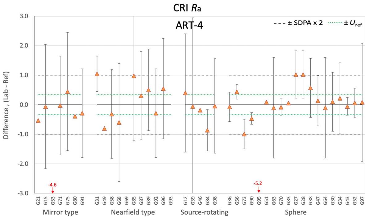
Figure 7-113. Differences of CRI  $R_a$  for ART-4 by goniophotometer type and sphere
