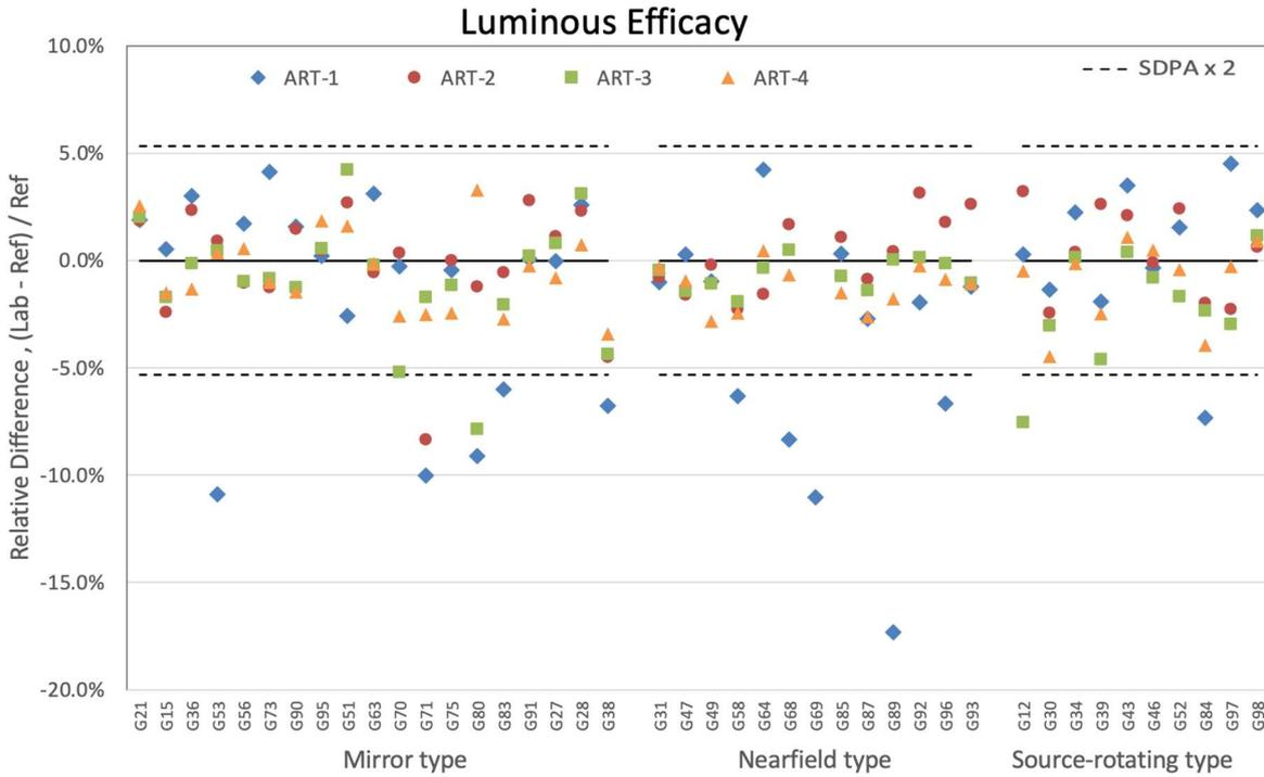
Figure 7-85. Relative differences of luminous efficacy for all artefacts by goniophotometer type
