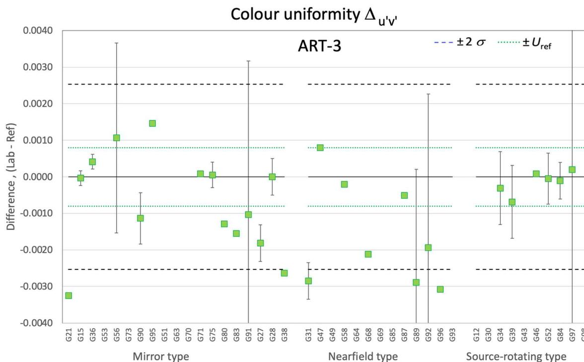
**Figure 7-126. Differences of colour uniformity for ART-3 by goniophotometer types**
