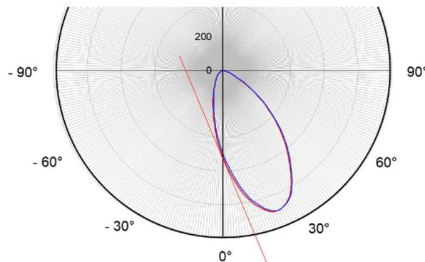
**Figure 7-69. Luminous intensity distribution of ART-4 in the plane perpendicular to road direction**
