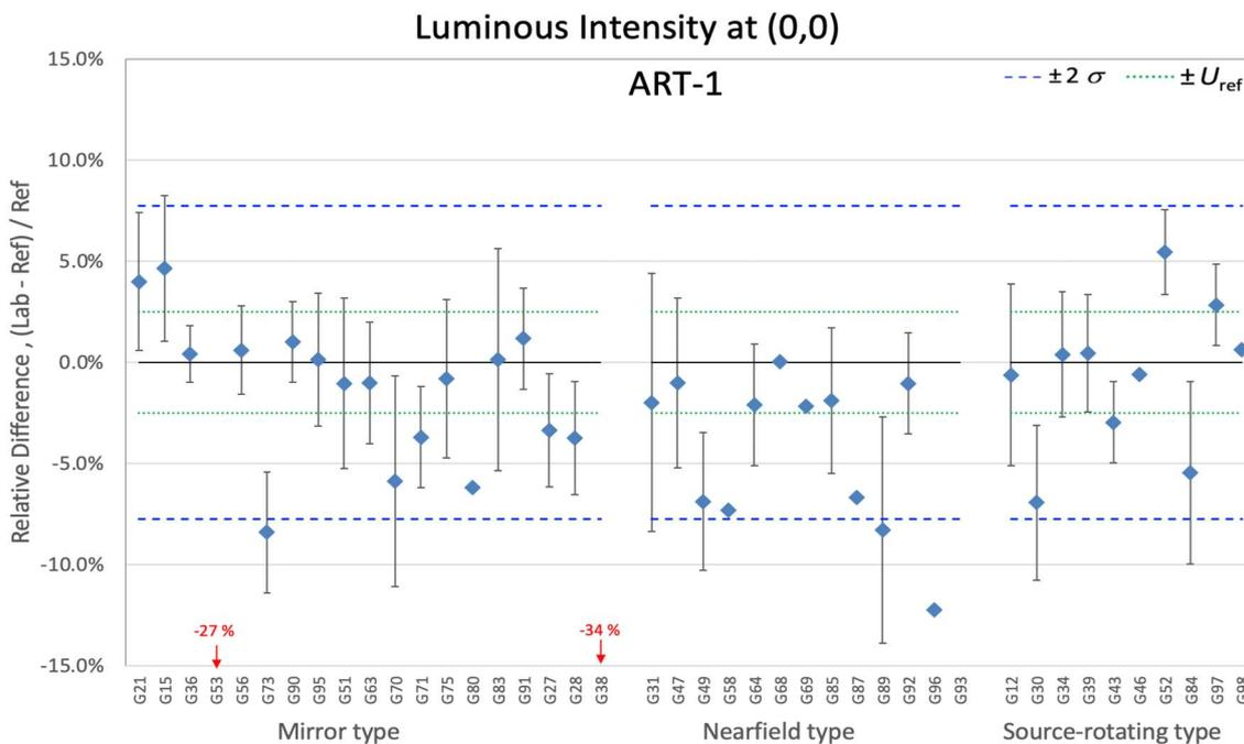
Figure 7-115. Relative differences of luminous intensity at (0,0) for ART-1 by goniophotometer type
