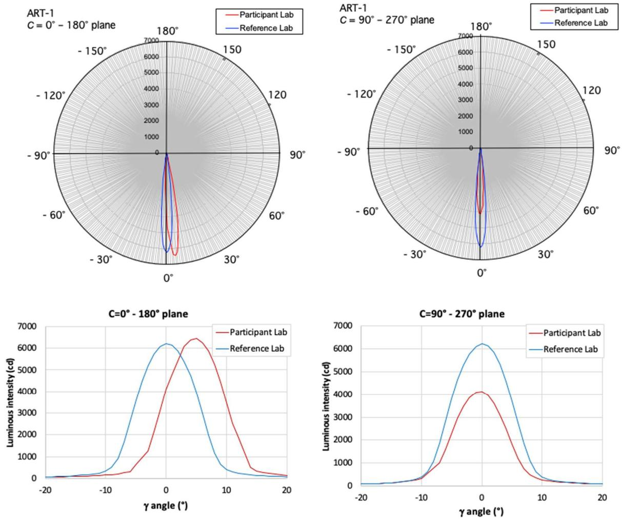
Figure 7-153. Example of a problem in poor alignment of the artefact (ART-1) (participant: mirror type goniophotometer)
