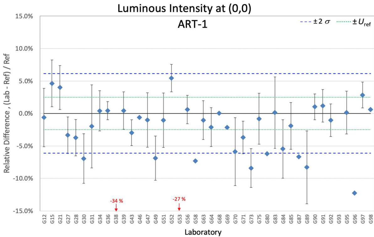
Figure 7-55. Relative differences of luminous intensity at (0,0) for ART-1
