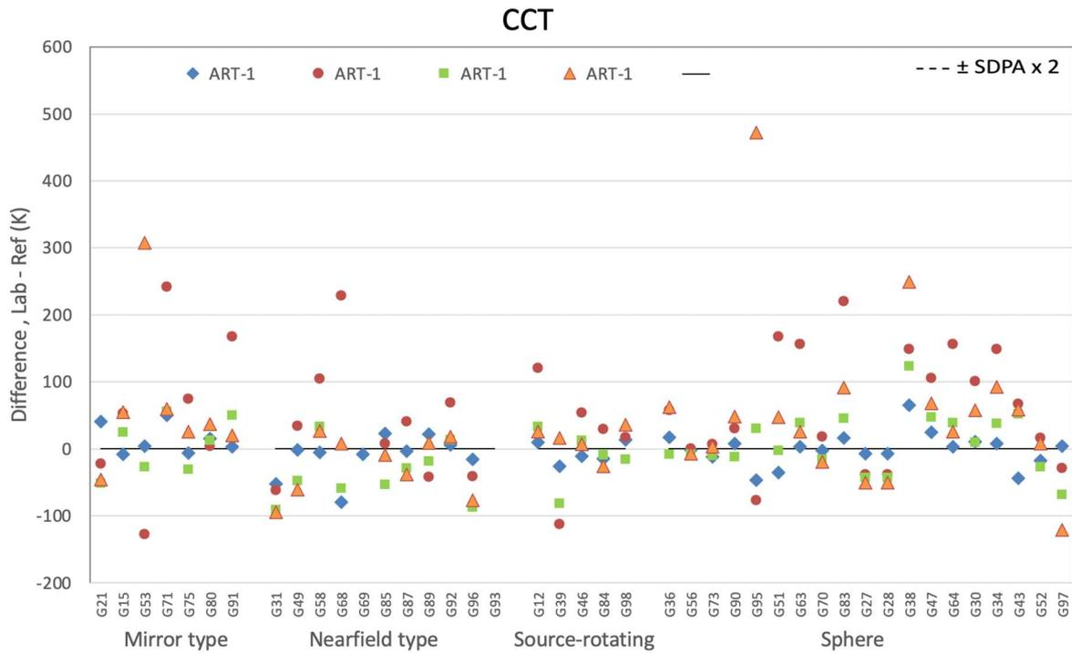
Figure 7-104. Differences of CCT for all artefacts by goniophotometer type and sphere
