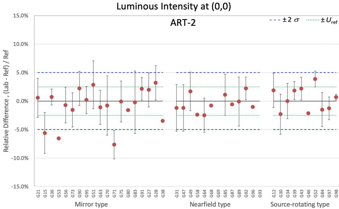
**Figure 7-116. Relative differences of luminous intensity at (0,0) for ART-2 by goniophotometer type**
