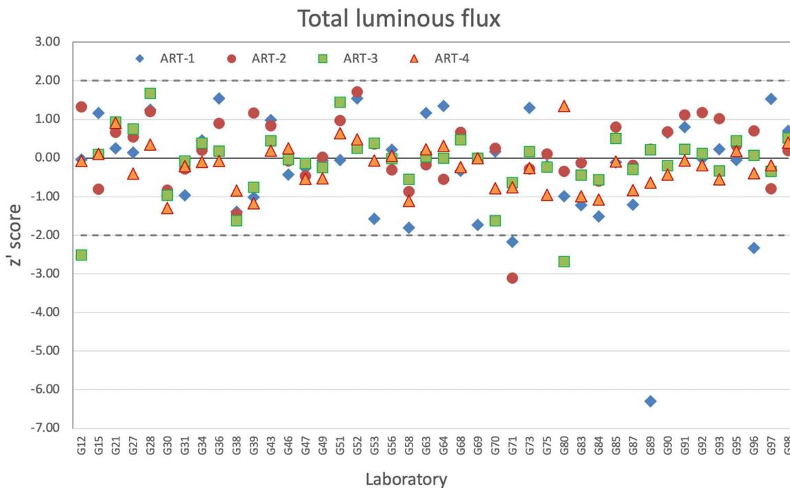
Figure 7-157.  $z'$  score results for total luminous flux for all artefacts
