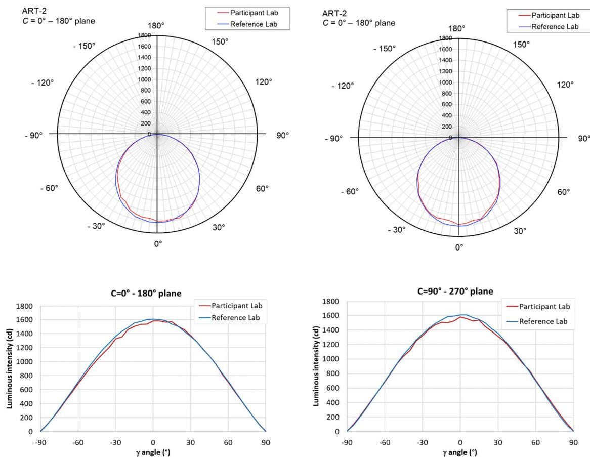
Figure 7-156. Example of noisy intensity distribution curves (ART-2) (participant: mirror type goniophotometer)
