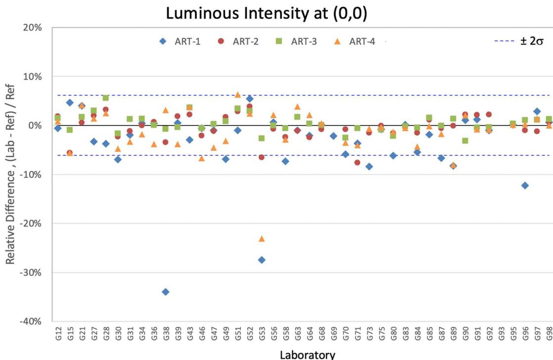
Figure 7-53. Relative differences of luminous intensity at (0,0) for all artefacts
