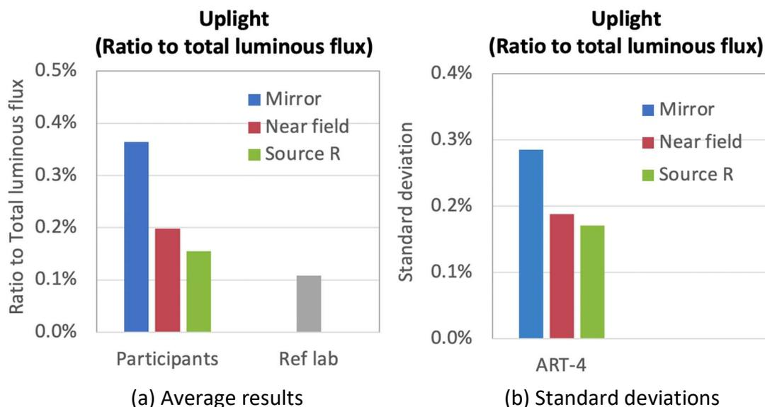
**Figure 7-144. The results of Uplight (ratio to total luminous flux) (a) and their standard deviations (b) for each instrument type**
