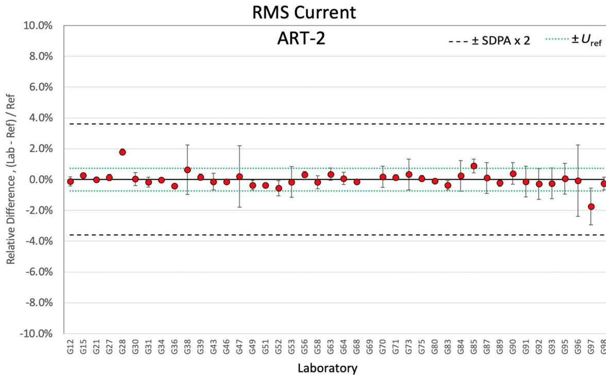
Figure 7-16. Relative differences of RMS current for ART-2
