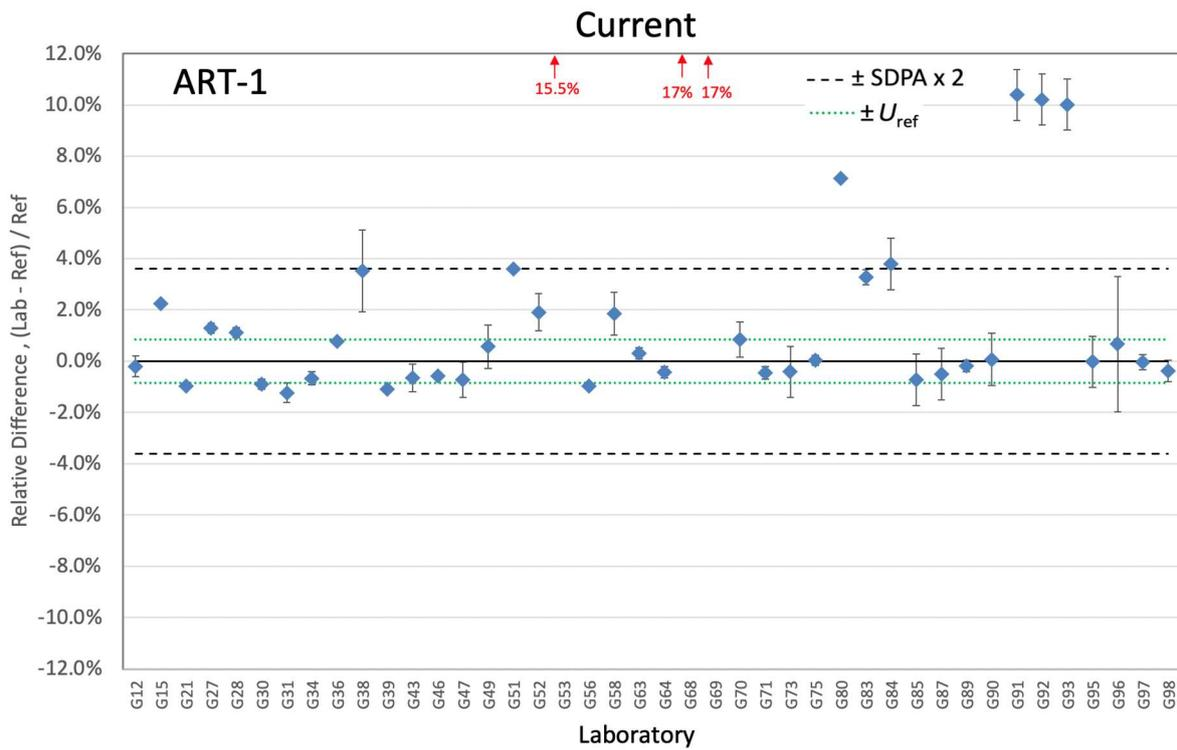
Figure 7-15. Relative differences of RMS current for ART-1
