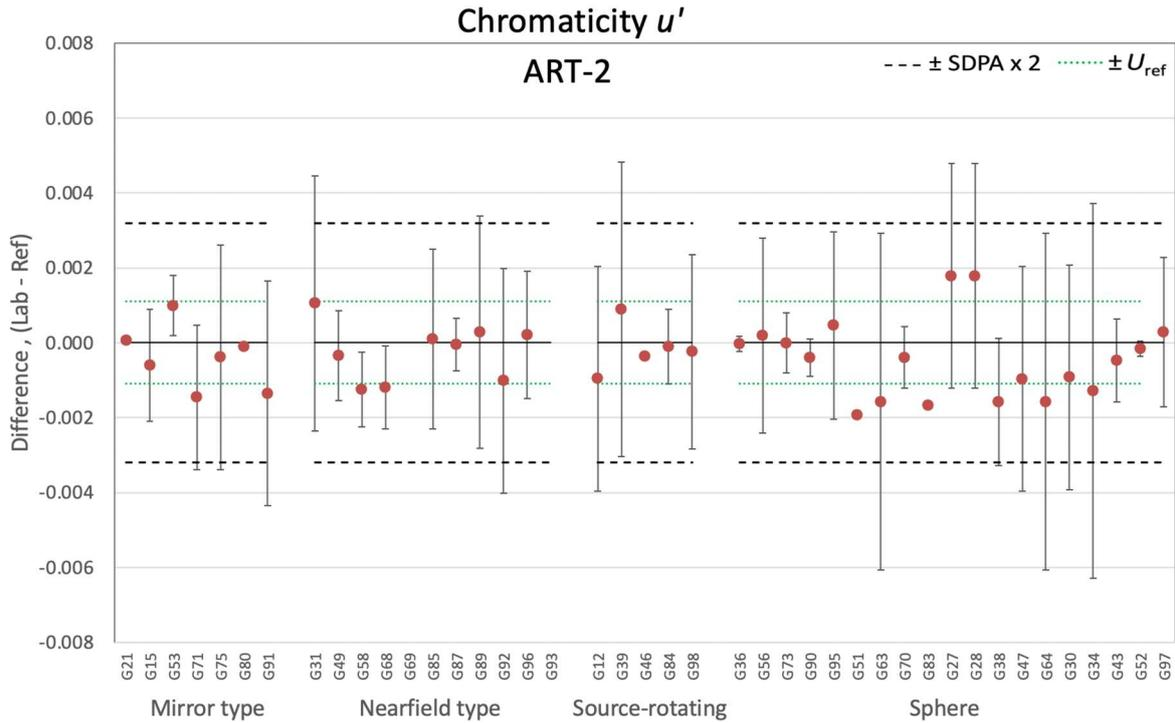
Figure 7-96. Differences of chromaticity  $u'$  for ART-2 by goniophotometer type and sphere
