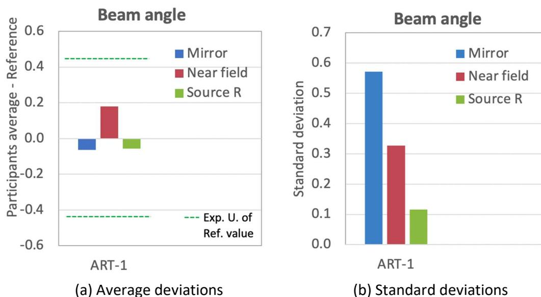
**Figure 7-141. Average deviations from the reference value (a) and the standard deviations (b) of beam angle for each instrument type**
