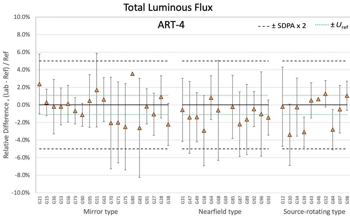
Figure 7-74. Relative differences of total luminous flux for ART-4 by goniophotometer type
