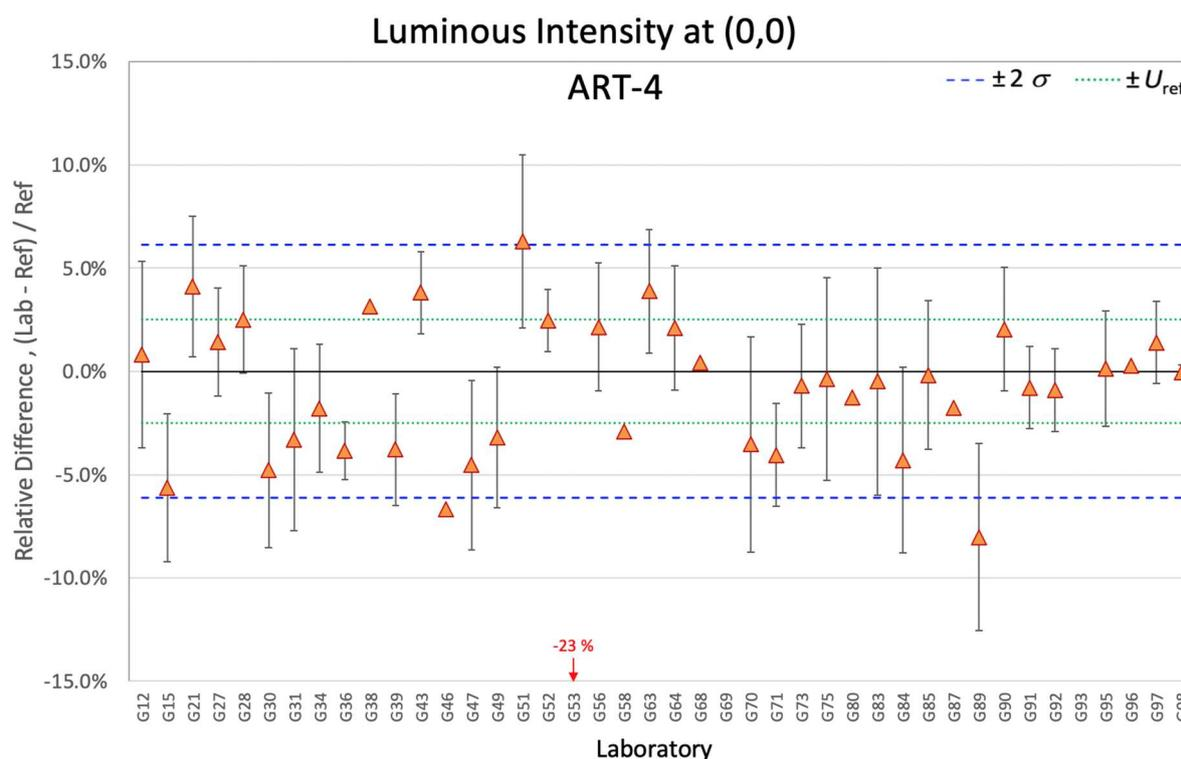
**Figure 7-58. Relative differences of luminous intensity at (0,0) for ART-4**
