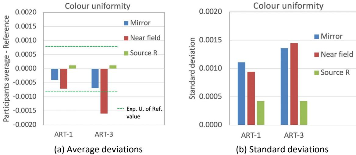
Figure 7-145. Average deviations from the reference value (a) and the standard deviations (b) of the results for colour uniformity for each instrument type
