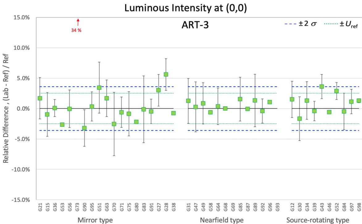
**Figure 7-117. Relative differences of luminous intensity at (0,0) for ART-3 by goniophotometer type**
