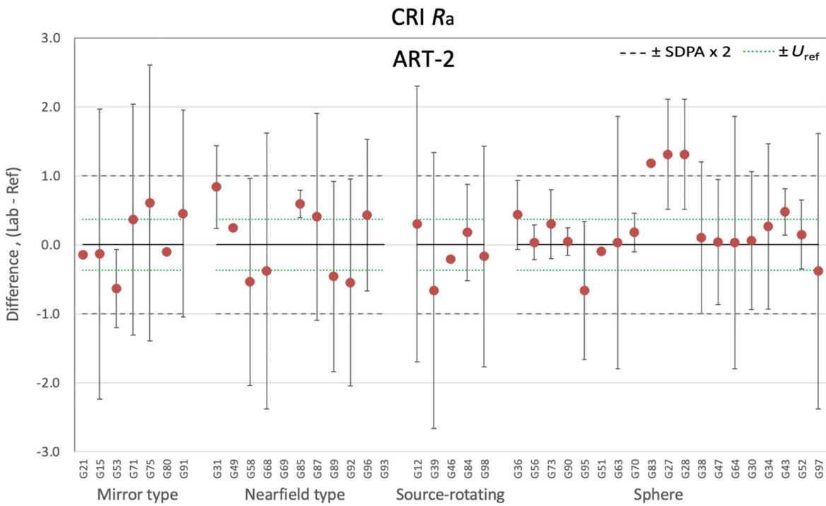
Figure 7-111. Differences of CRI  $R_a$  for ART-2 by goniophotometer type and sphere
