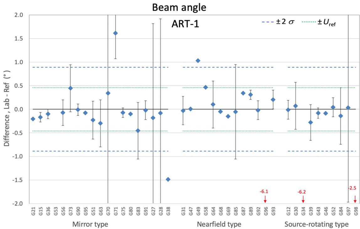
Figure 7-121. Differences of beam angle for ART-1 by goniophotometer type
