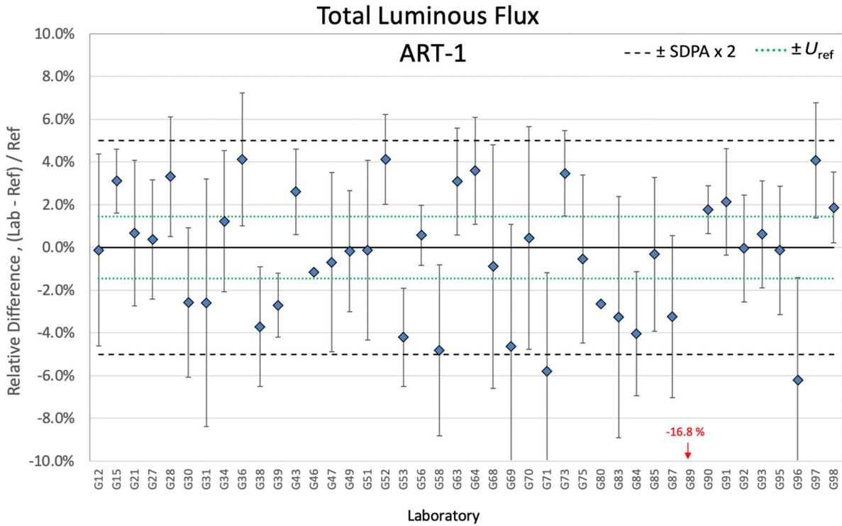
**Figure 7-3. Relative differences of total luminous flux for ART-1**
