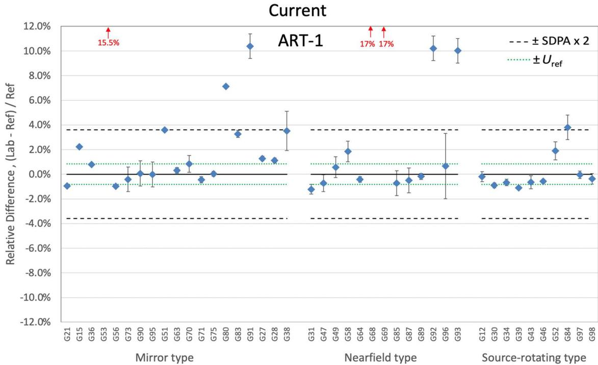
Figure 7-81. Relative differences of RMS current for ART-1 by goniophotometer type
