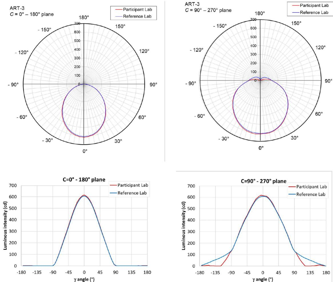
**Figure 7-155. Example of a problem in dead angle of the goniophotometer for ART-3 (Participant’s curve beyond  $\gamma = \pm 150^\circ$  is shadowed) (participant: source-rotating type goniophotometer)**
