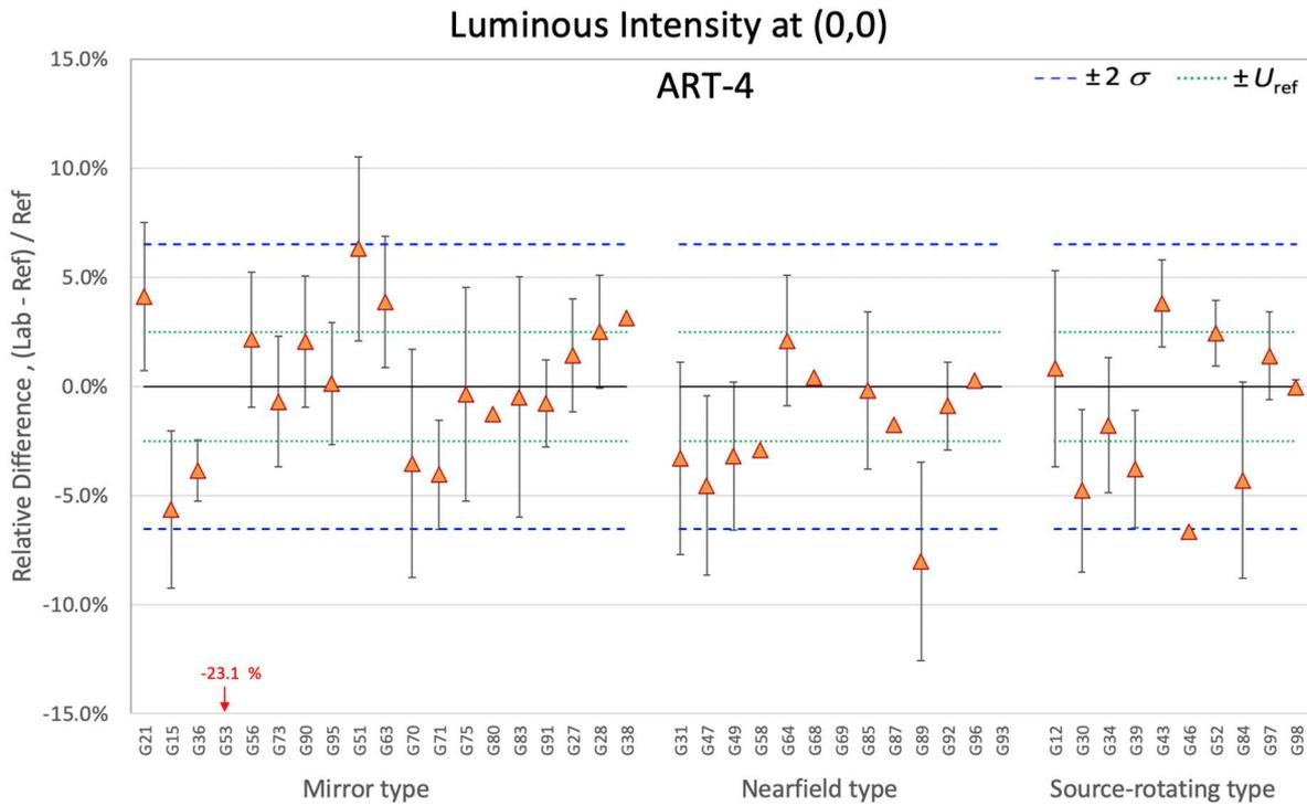
**Figure 7-118. Relative differences of luminous intensity at (0,0) for ART-4 by goniophotometer type**
