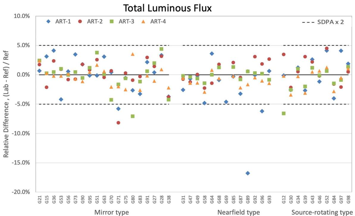
**Figure 7-70. Relative differences of total luminous flux for all artefacts sorted by goniophotometer type**
