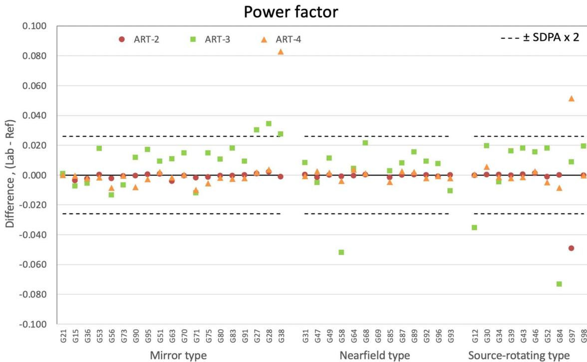
**Figure 7-90. Differences of power factor for all artefacts by goniophotometer type (ART-1 was DC, not included)**
