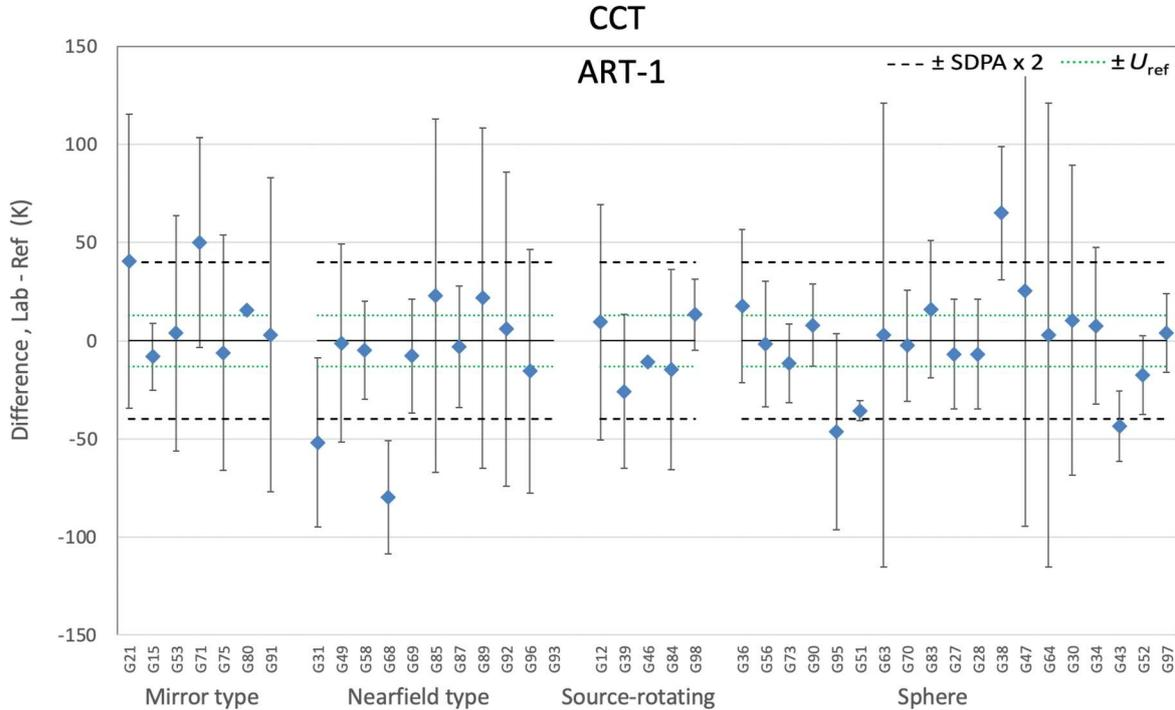
Figure 7-105. Differences of CCT for ART-1 by goniophotometer type and sphere
