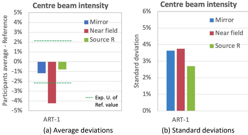
**Figure 7-139. Average deviations from the reference value (a) and the standard deviations (b) deviations of centre beam intensity results for each instrument type**
