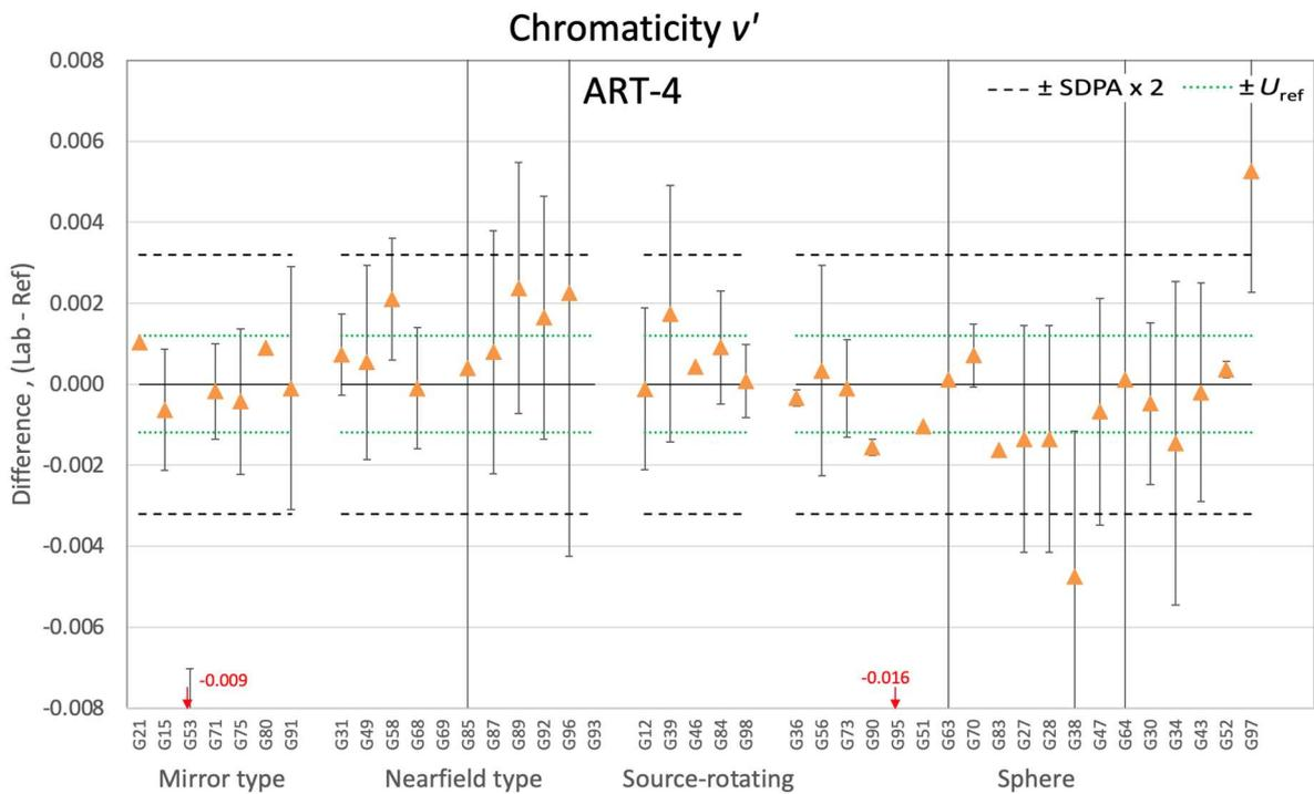
Figure 7-103. Differences of chromaticity  $v'$  for ART-4 by goniophotometer type and sphere
