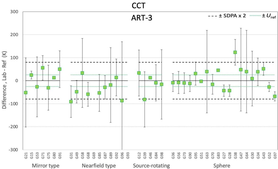
Figure 7-107. Differences of CCT for ART-3 by goniophotometer type and sphere
