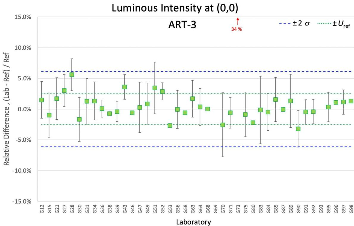
**Figure 7-57. Relative differences of luminous intensity at (0,0) for ART-3**
