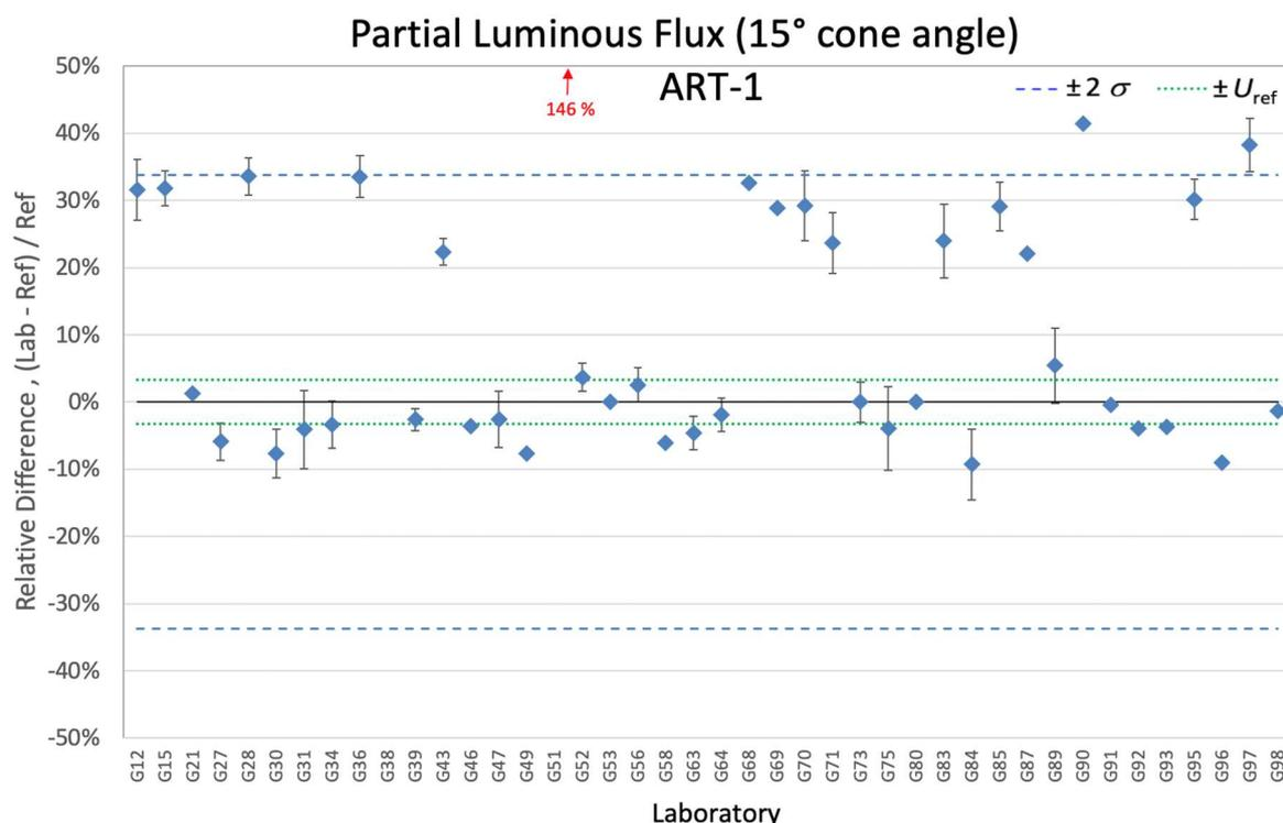
**Figure 7-60. Relative differences of partial luminous flux for ART-1**
