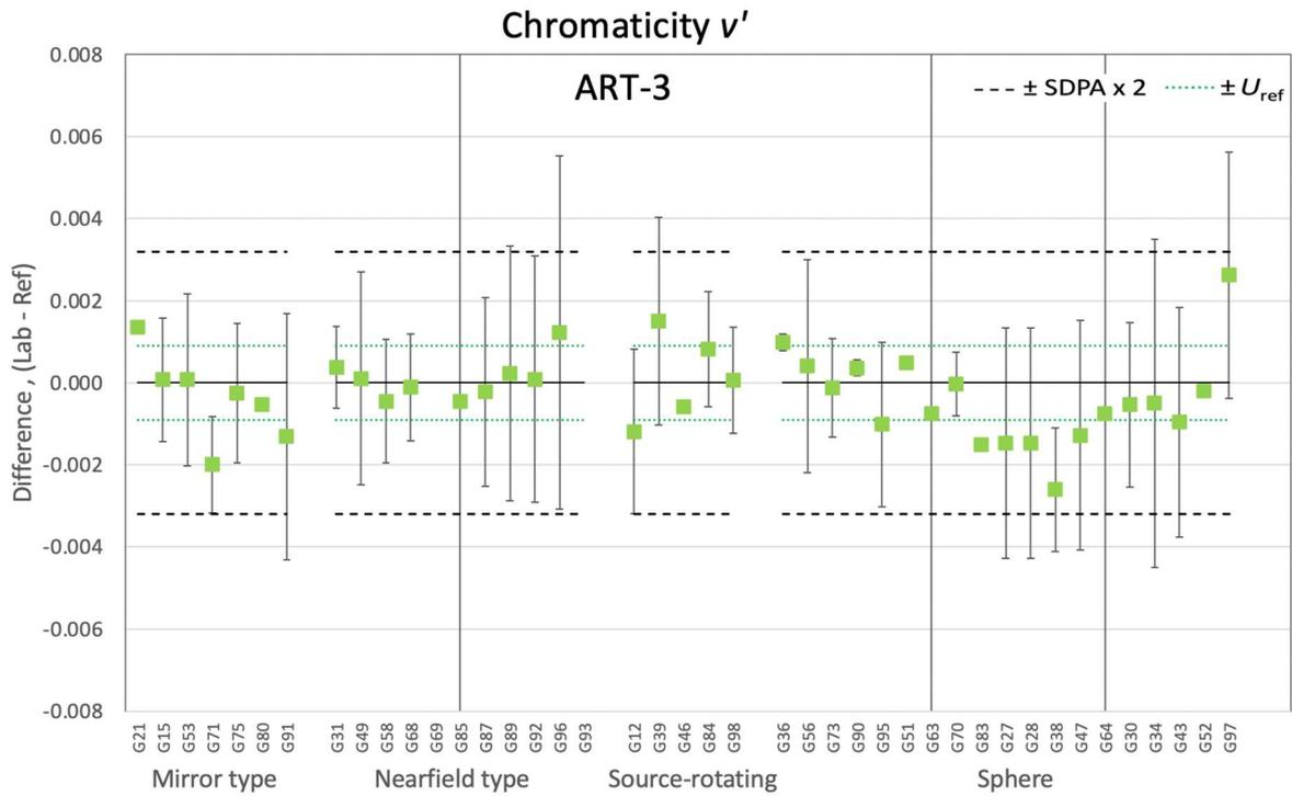
Figure 7-102. Differences of chromaticity  $v'$  for ART-3 by goniophotometer type and sphere
