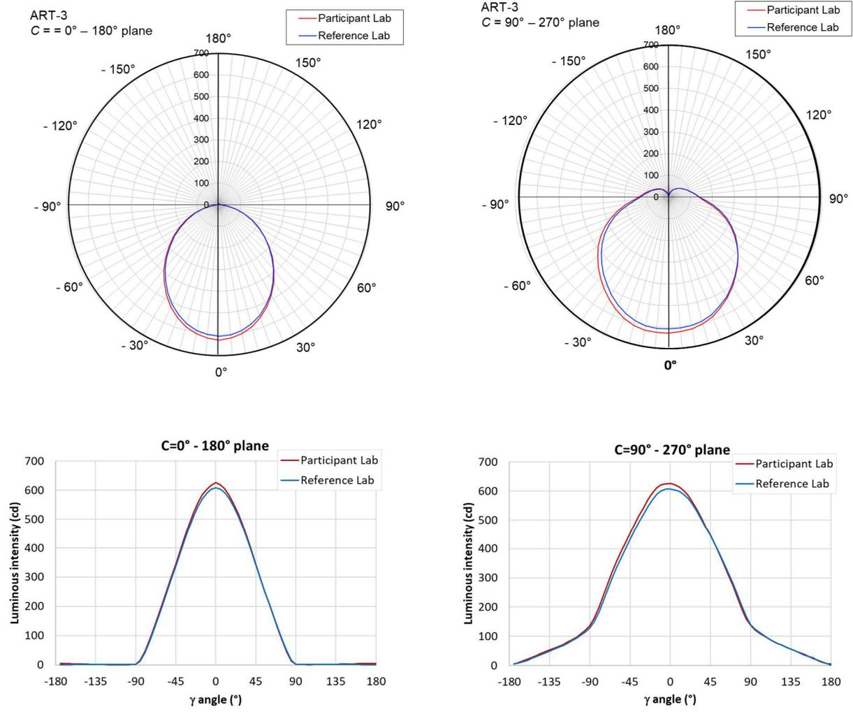
**Figure 7-149. Example of luminous intensity distribution comparison of ART-3 (participant: mirror type goniophotometer)**
