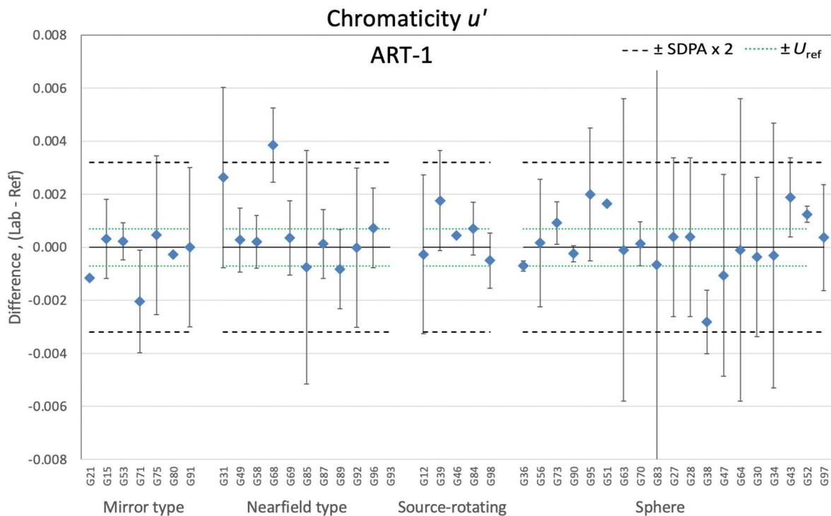
Figure 7-95. Differences of chromaticity  $u'$  for ART-1 by goniophotometer type and sphere
