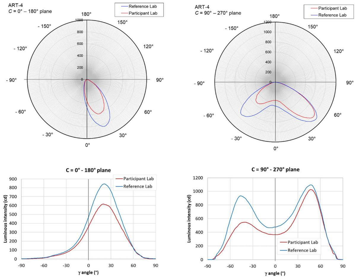
**Figure 7-154. Example of a problem in poor alignment of the artefact (ART-4) (participant: mirror type goniophotometer)**
