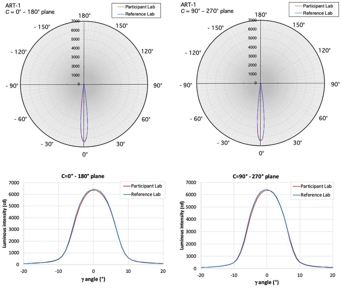
**Figure 7-151. Example of luminous intensity distribution comparison of ART-1 (participant: near-field goniophotometer)**
