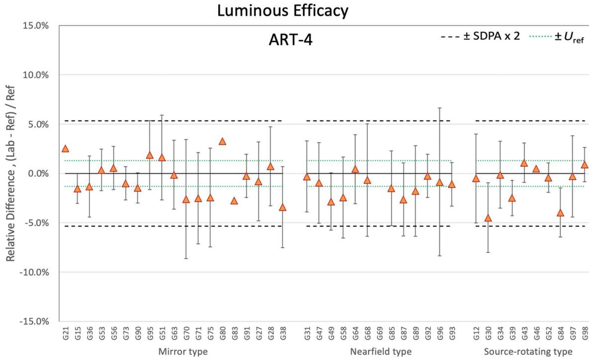
**Figure 7-89. Relative differences of luminous efficacy for ART-4 by goniophotometer type**
