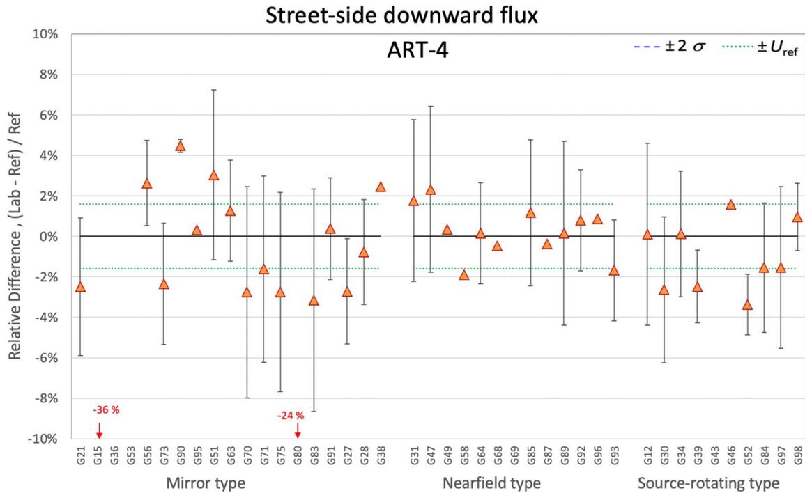
**Figure 7-122. Relative differences of Street-side downward flux for ART-4 by goniophotometer type**
