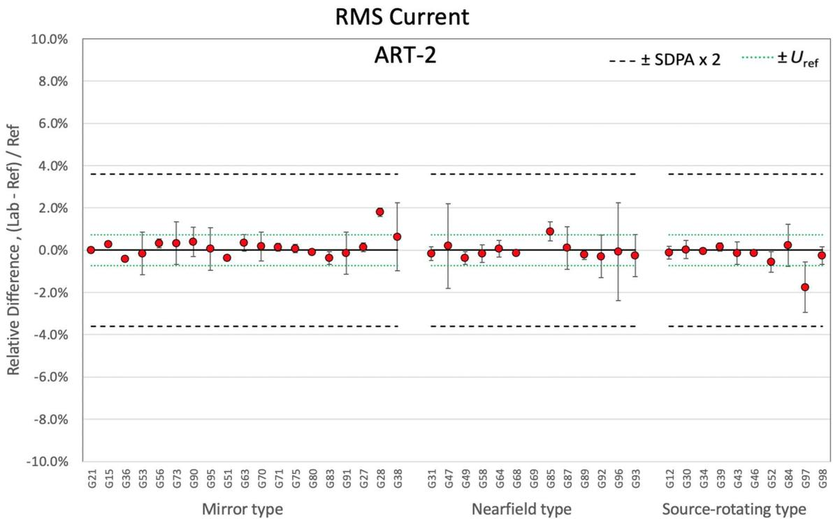
Figure 7-82. Relative differences of RMS current for ART-2 by goniophotometer type
