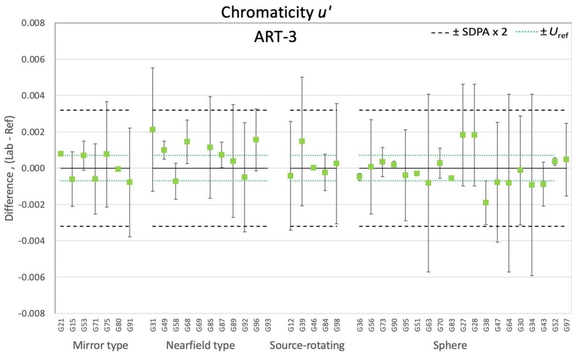
Figure 7-97. Differences of chromaticity  $u'$  for ART-3 by goniophotometer type and sphere
