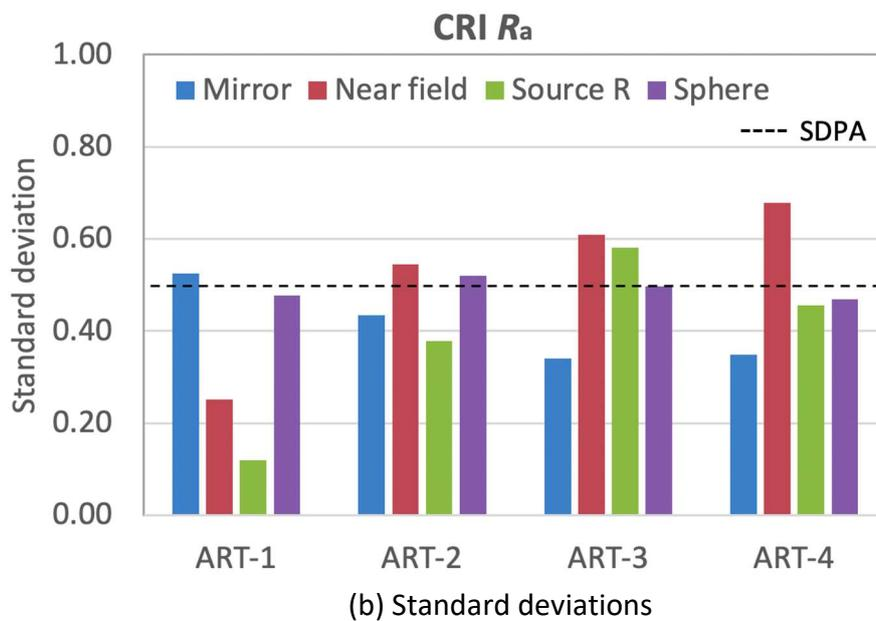
**Figure 7-137. Average deviations from the reference value (a) and the standard deviations (b) of CRI  $R_a$  results for sphere and gonio**
