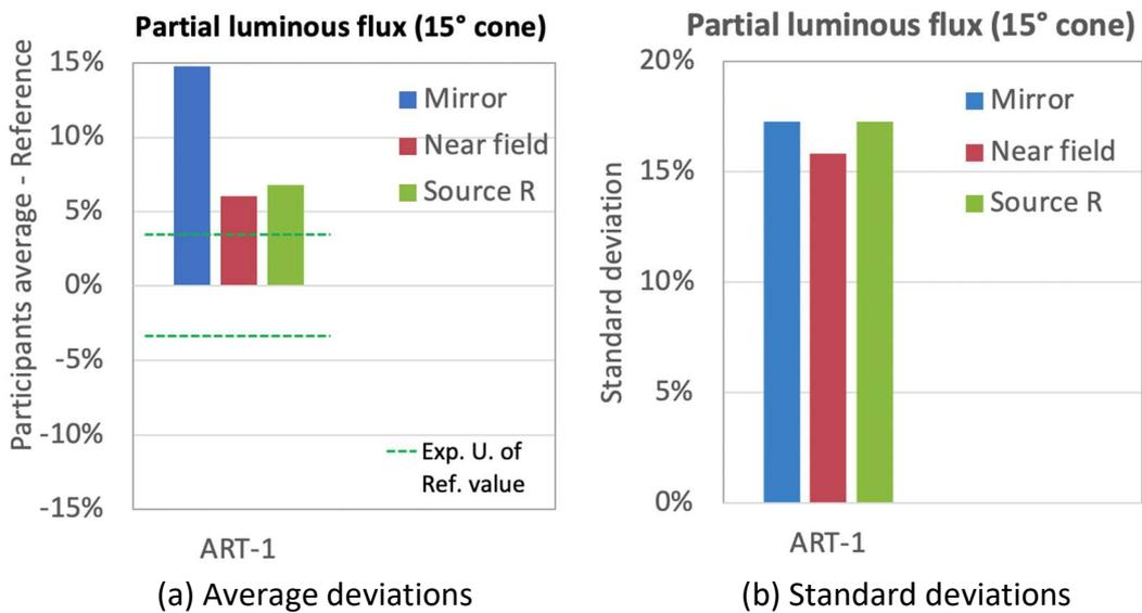
**Figure 7-140. Average deviations from the reference value (a) and the standard deviations (b) of the results of partial luminous flux (15° cone) for each instrument type**
