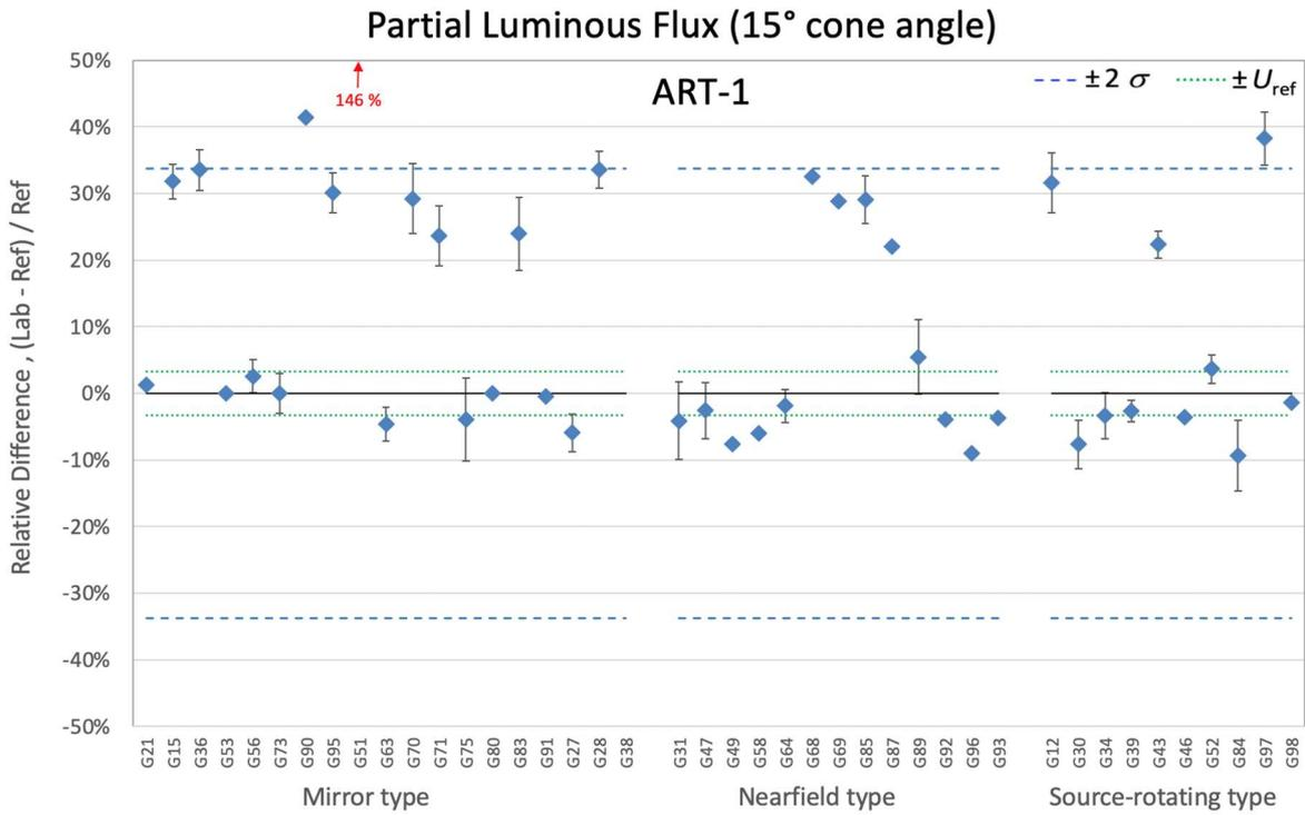
Figure 7-120. Relative differences of partial luminous flux for ART-1 by goniophotometer type
