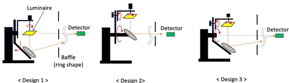
**Figure A1-2. Three variations of the mirror type goniophotometer design**
