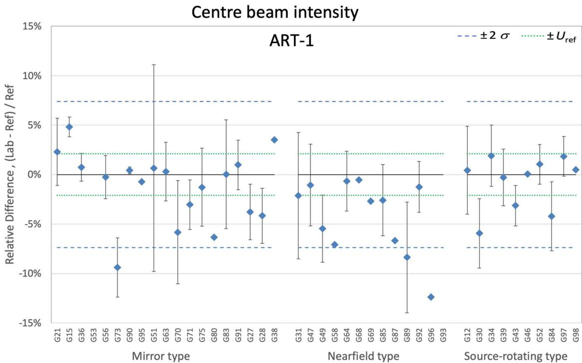
**Figure 7-119. Relative differences of centre beam intensity for ART-1 by goniophotometer type**
