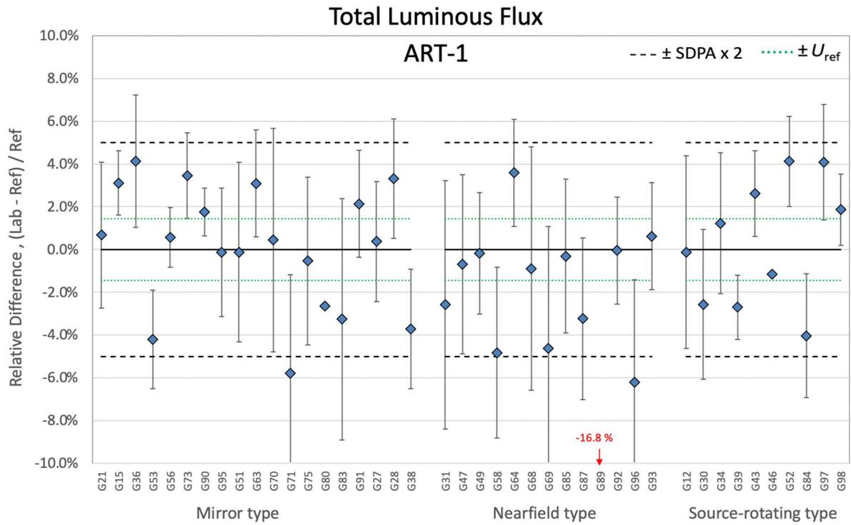
**Figure 7-71. Relative differences of total luminous flux for ART-1 by goniophotometer type**
