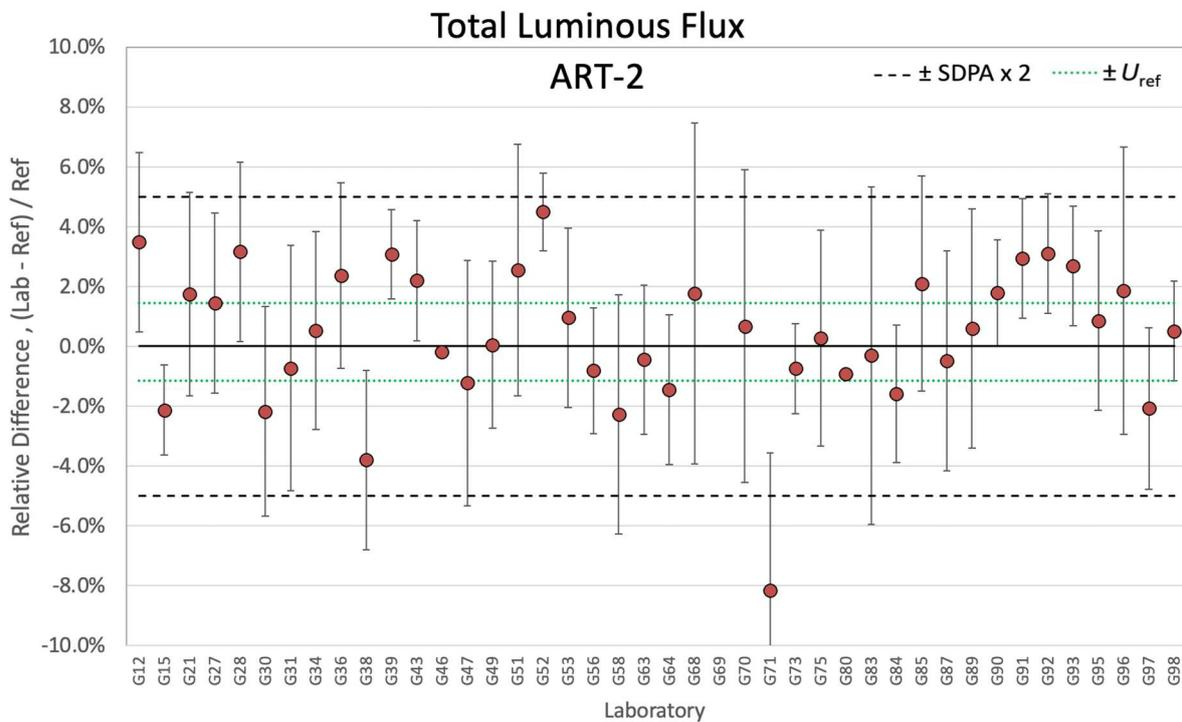
**Figure 7-4. Relative differences of total luminous flux for ART-2**
