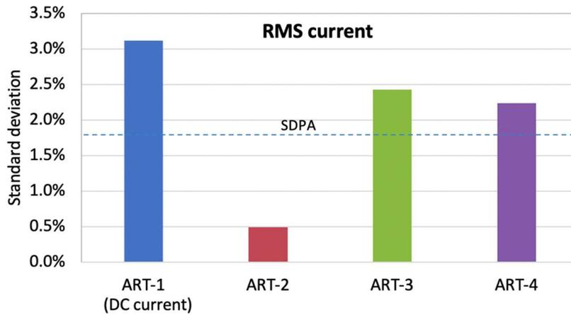
Figure 7-14. Relative standard deviations of RMS current results
