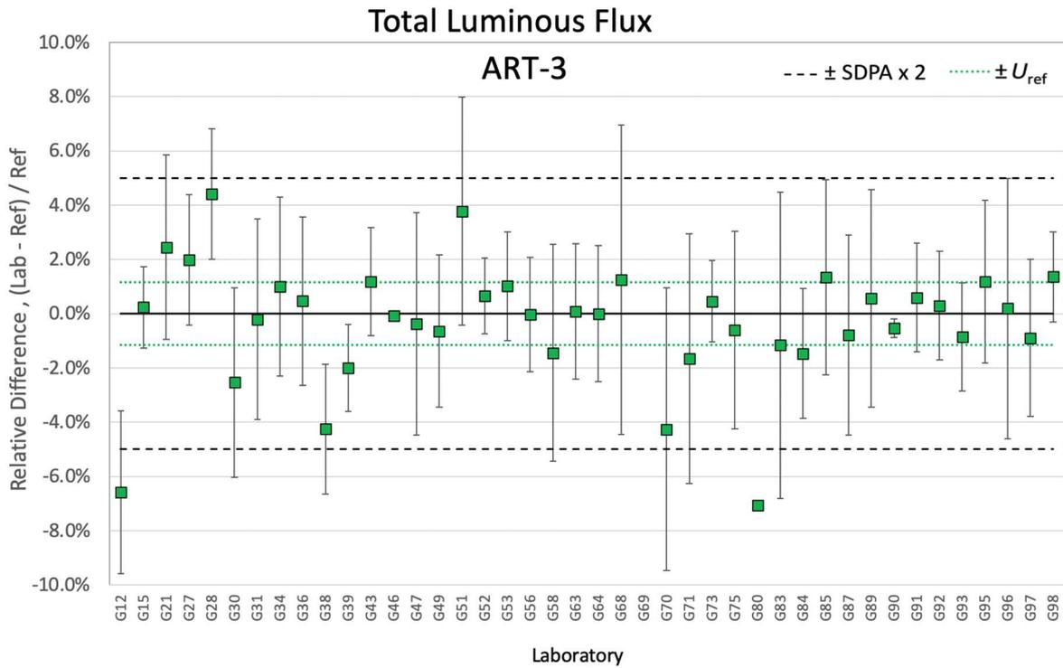
Figure 7-5. Relative differences of total luminous flux for ART-3
