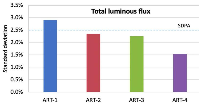
Figure 7-2. Relative standard deviations of total luminous flux results
