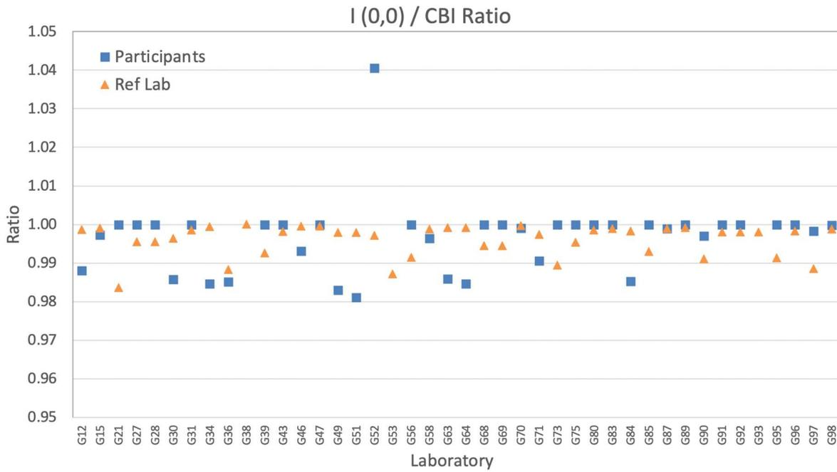
**Figure 7-68. The ratios of luminous intensity at (0,0) to centre beam intensity (CBI) measured by each participant laboratory and reference laboratory.**
