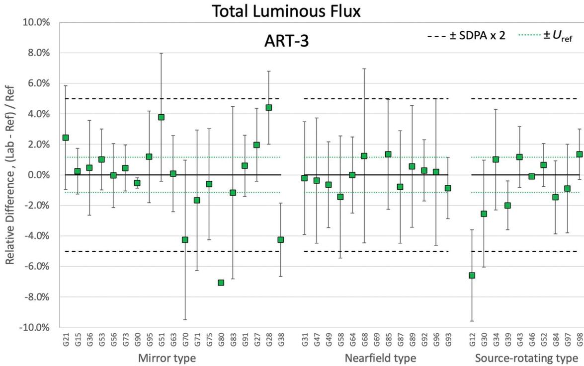
Figure 7-73. Relative differences of total luminous flux for ART-3 by goniophotometer type
