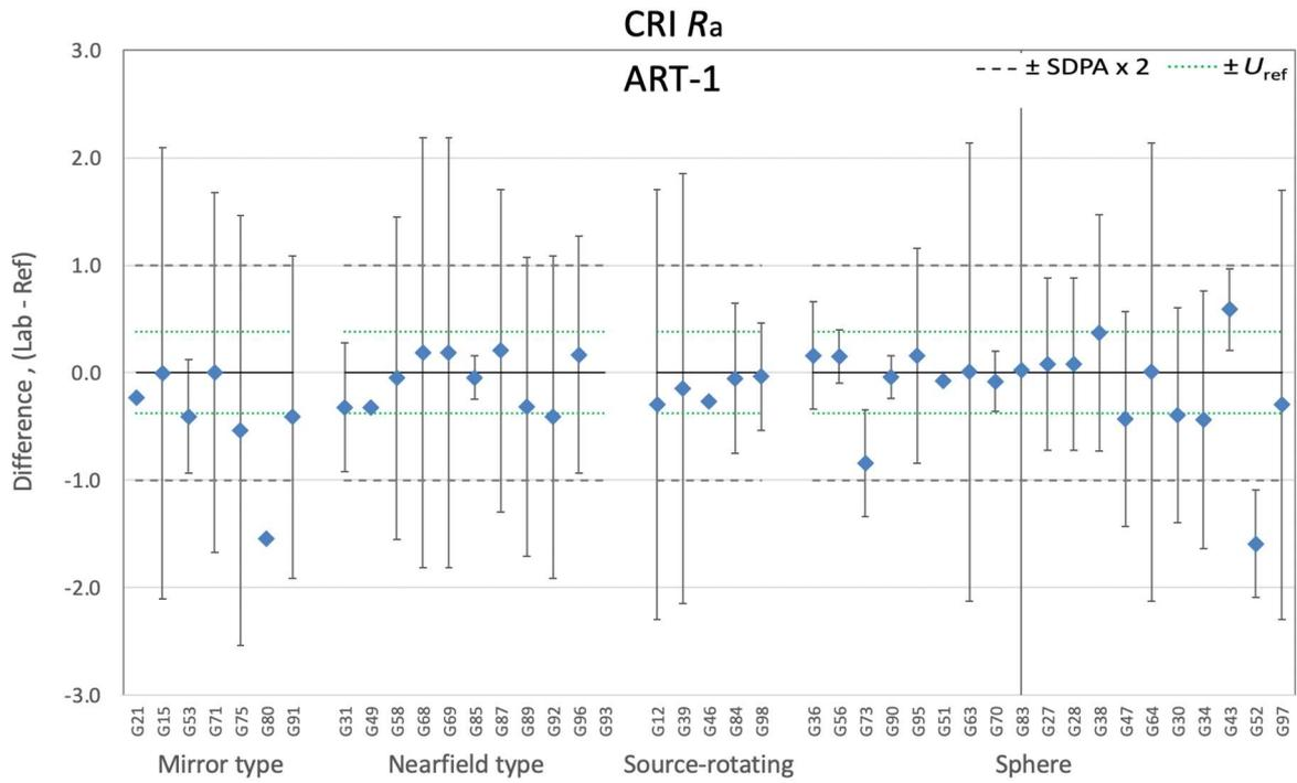
Figure 7-110. Differences of CRI  $R_a$  for ART-1 by goniophotometer type and sphere
