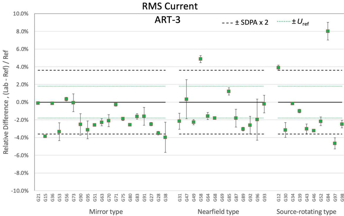
Figure 7-83. Relative differences of RMS current for ART-3 by goniophotometer type
