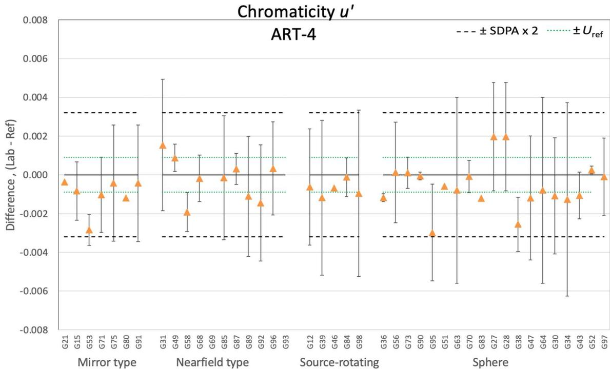
**Figure 7-98. Differences of chromaticity  $u'$  for ART-4 by goniophotometer type and sphere**
