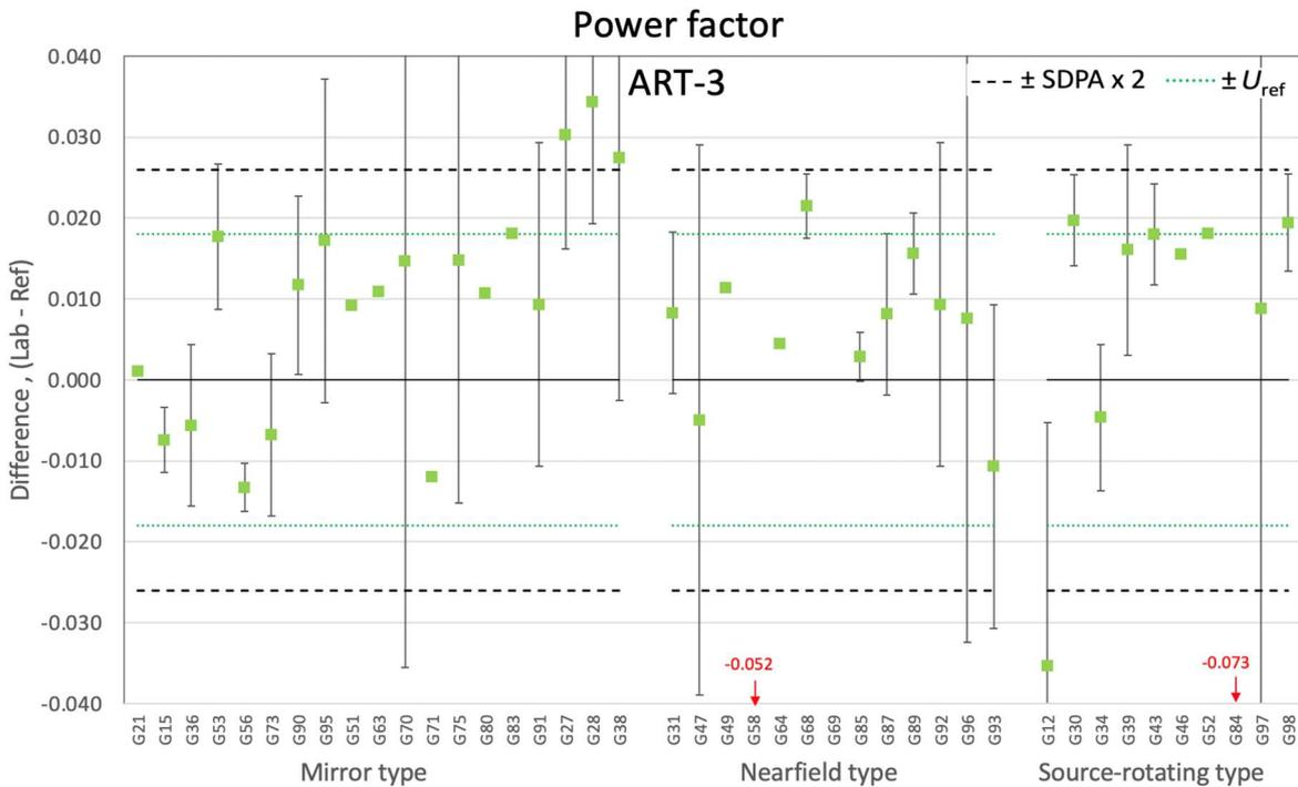
Figure 7-92. Differences of power factor for ART-3 by goniophotometer type
