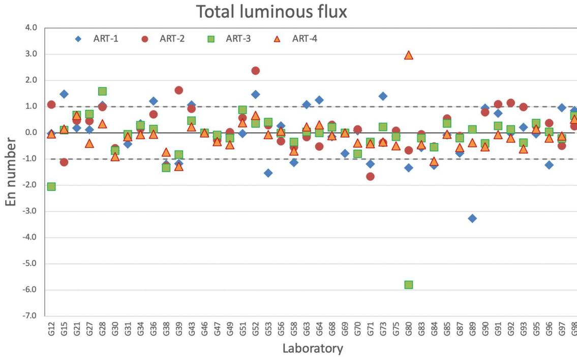
**Figure 7-158. E<sub>n</sub> number results for total luminous flux for all artefacts**
