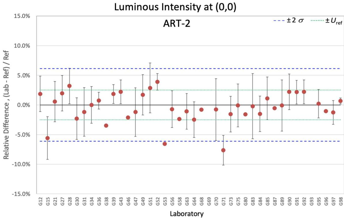
**Figure 7-56. Relative differences of luminous intensity at (0,0) for ART-2**
