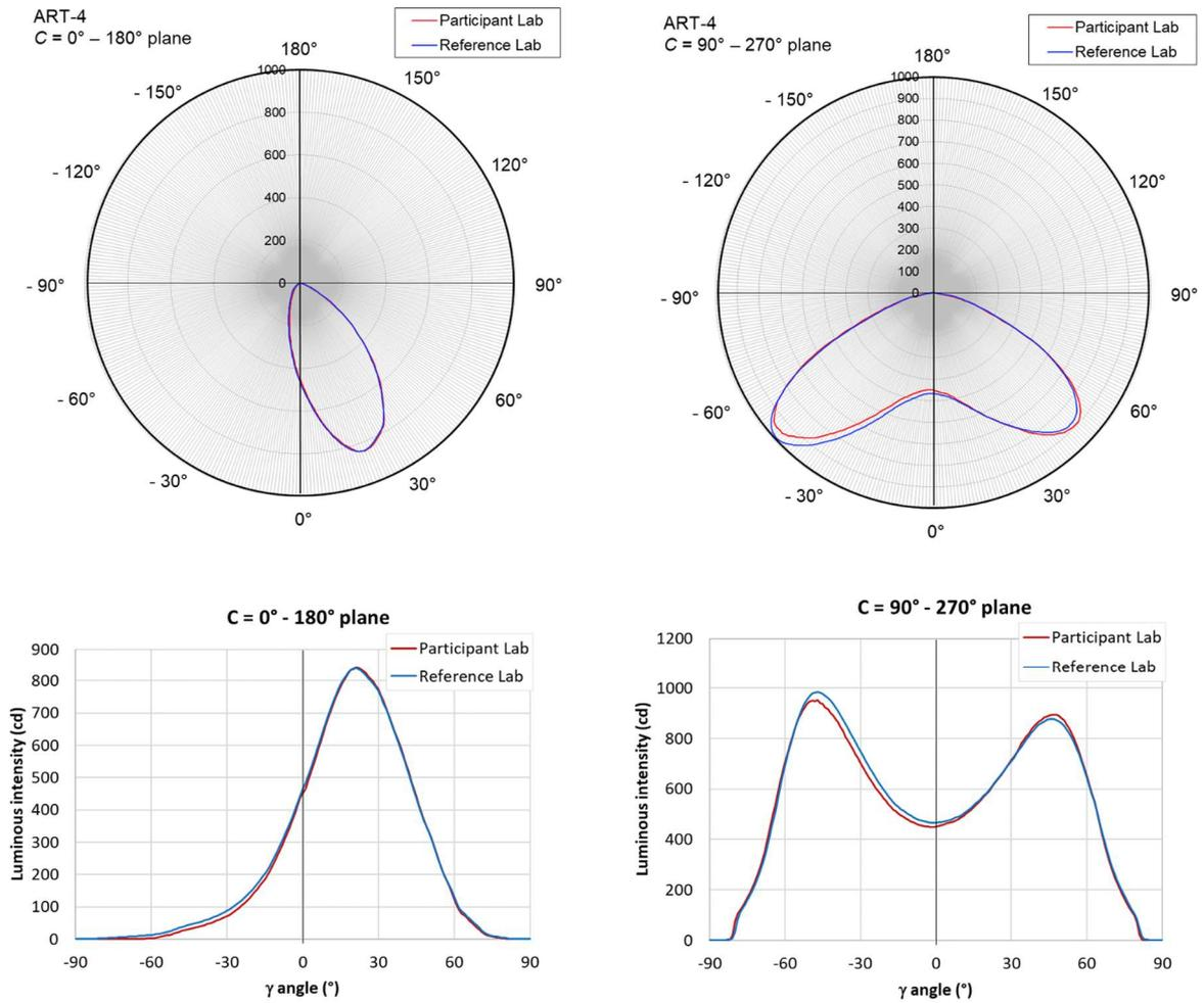
**Figure 7-152. Example of luminous intensity distribution comparison of ART-4 (participant: near-field goniophotometer)**
