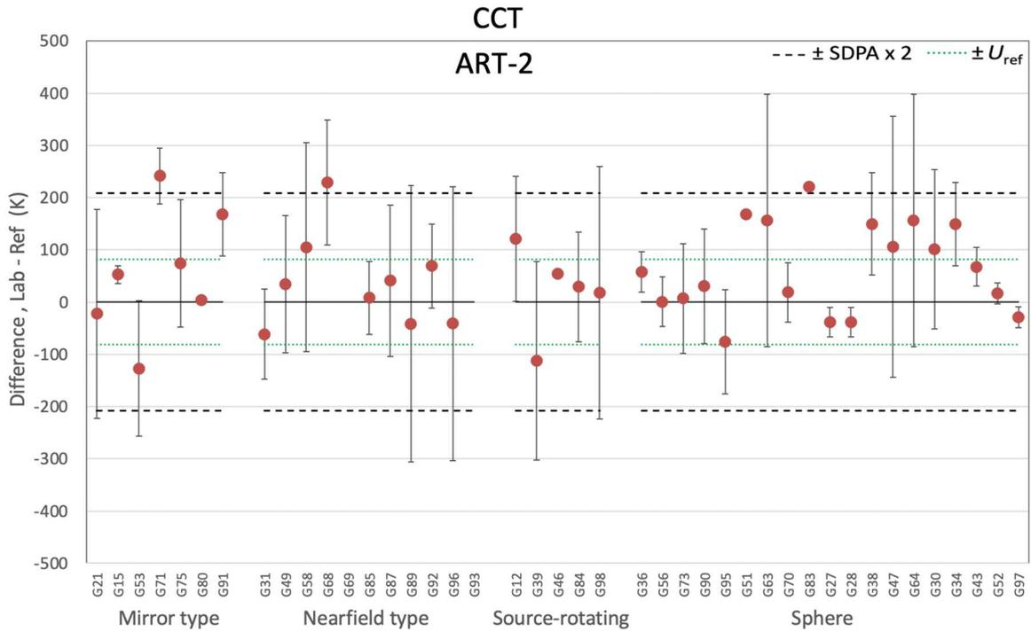
Figure 7-106. Differences of CCT for ART-2 by goniophotometer type and sphere
