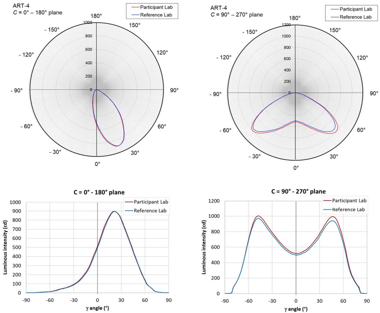
**Figure 7-150. Example of luminous intensity distribution comparison of ART-4 (participant: source-rotating type goniophotometer)**
