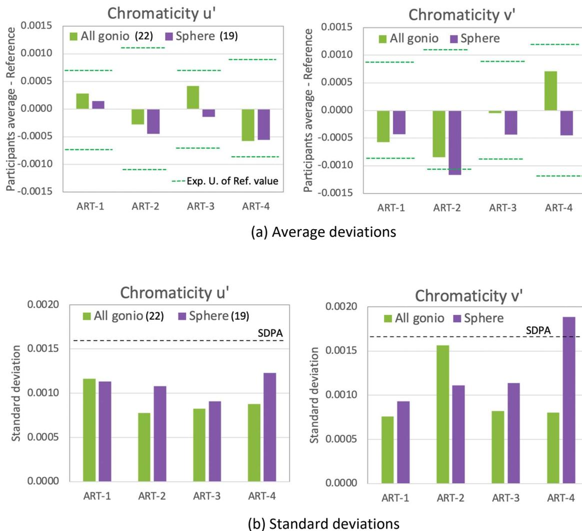
**Figure 7-135. Average deviations from the reference value (a) and the standard deviations (b) of chromaticity results for sphere and all goniophotometers**
