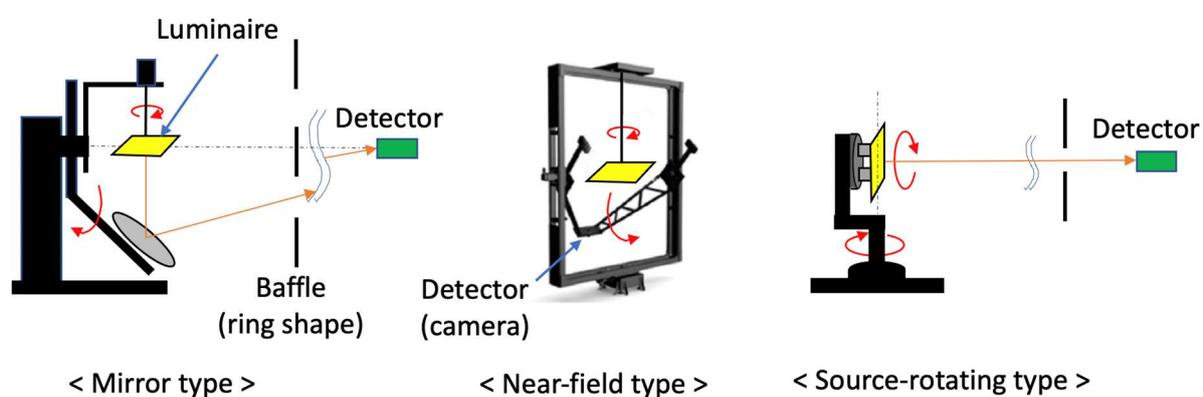
Figure A1-1. Schematics of three types of goniophotometers covered in IC 2017
