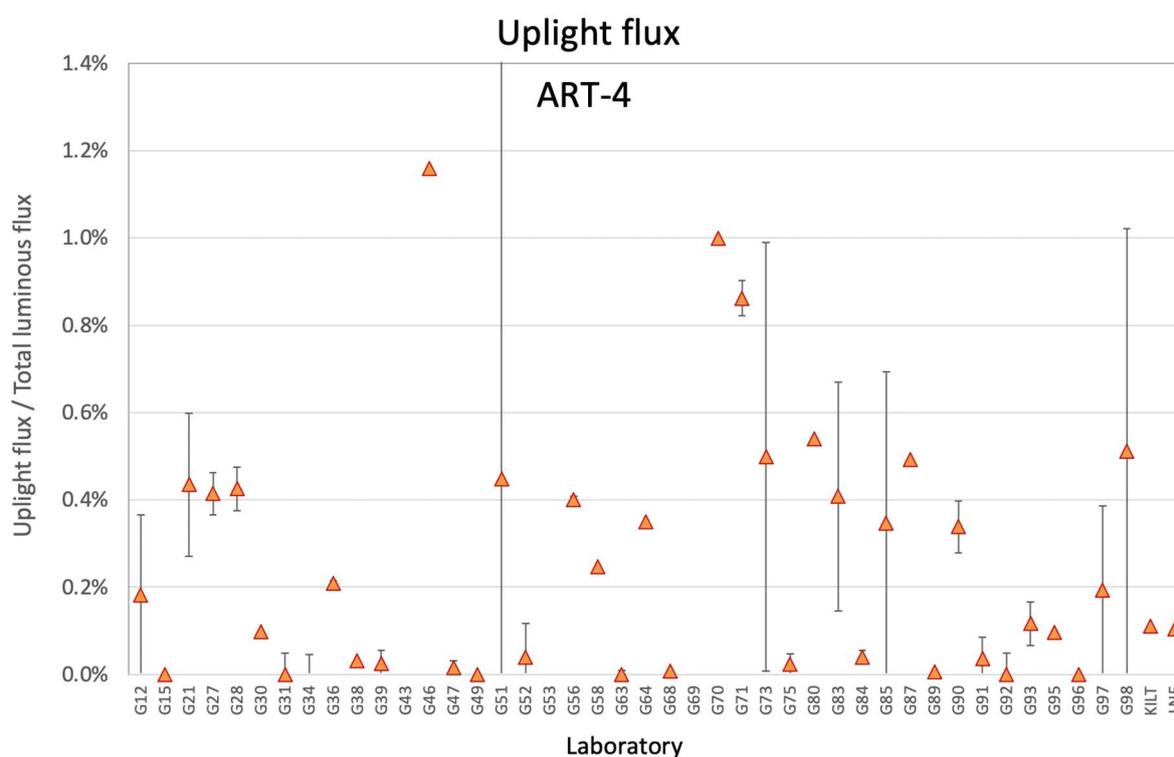
**Figure 7-64. Uplight flux relative to total luminous flux for ART-4**
