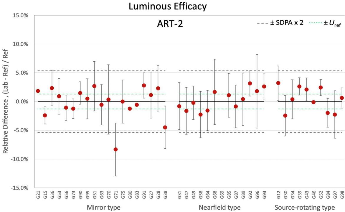
Figure 7-87. Relative differences of luminous efficacy for ART-2 by goniophotometer type
