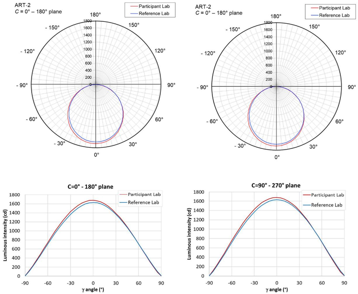
**Figure 7-148. Example of luminous intensity distribution comparison of ART-2 (participant: mirror type goniophotometer)**
