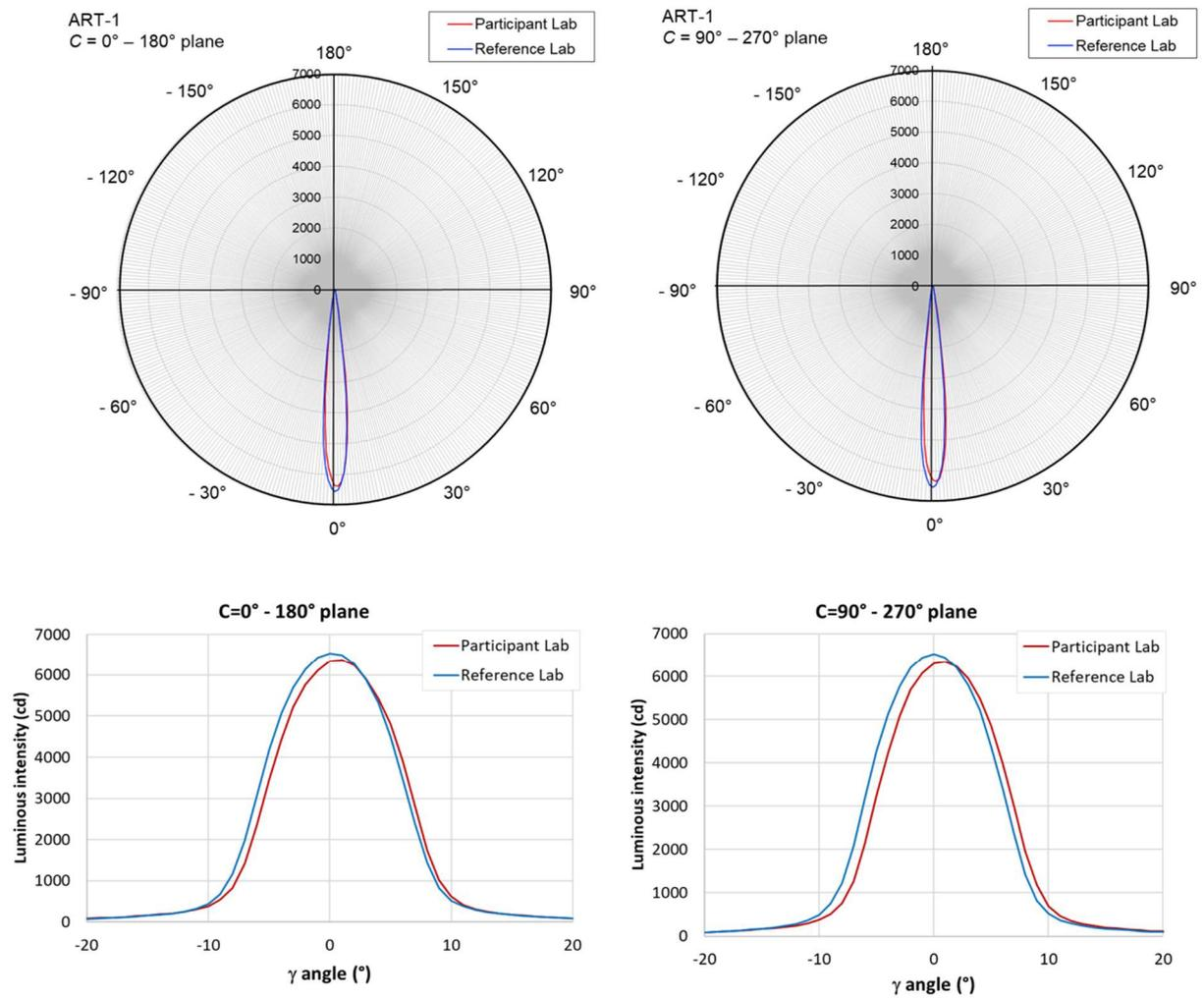
Figure 7-147. Example of luminous intensity distribution comparison of ART-1 (participant: source-rotating type goniophotometer)
