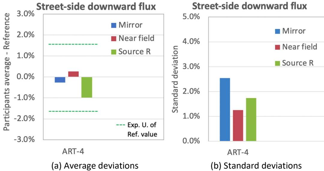
**Figure 7-142. Average deviations from the reference value (a) and the standard deviations (b) of the results of Street-side downward flux for each instrument type**
