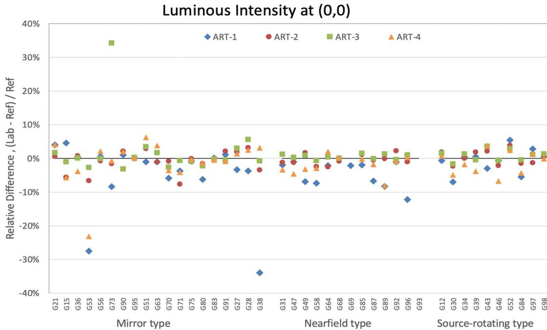
Figure 7-114. Relative differences of luminous intensity at (0,0) for all artefacts by goniophotometer type
