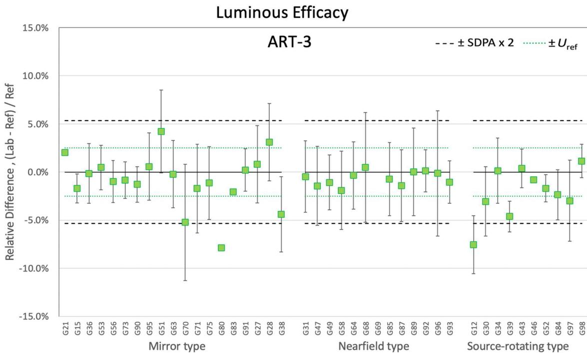
Figure 7-88. Relative differences of luminous efficacy for ART-3 by goniophotometer type
