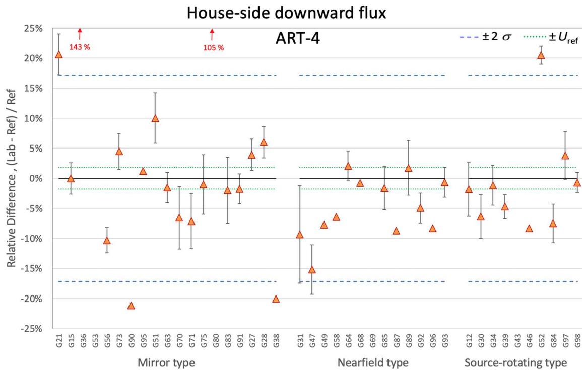
**Figure 7-123. Relative differences of House-side downward flux for ART-4 by goniophotometer type**
