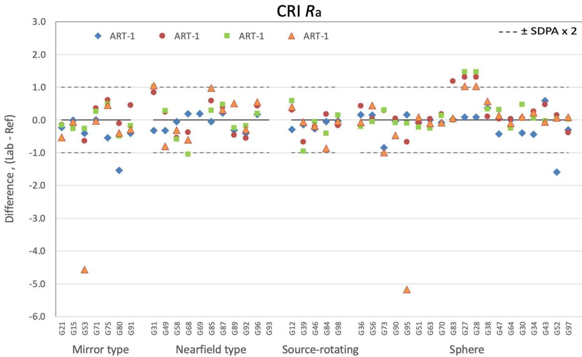
Figure 7-109. Differences of CRI Ra for all artefacts by goniophotometer type and sphere
