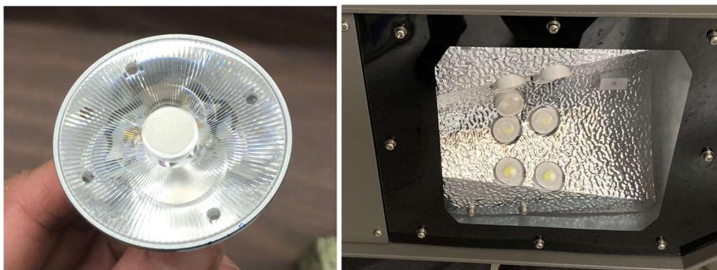
Figure 3-1. Light-emitting areas of ART-1 lamp (left) and ART-4 street lighting luminaire (right)
