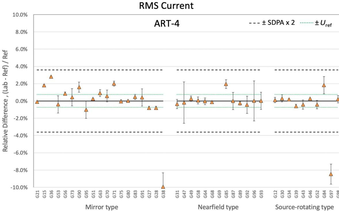
Figure 7-84. Relative differences of RMS current for ART-4 by goniophotometer type
