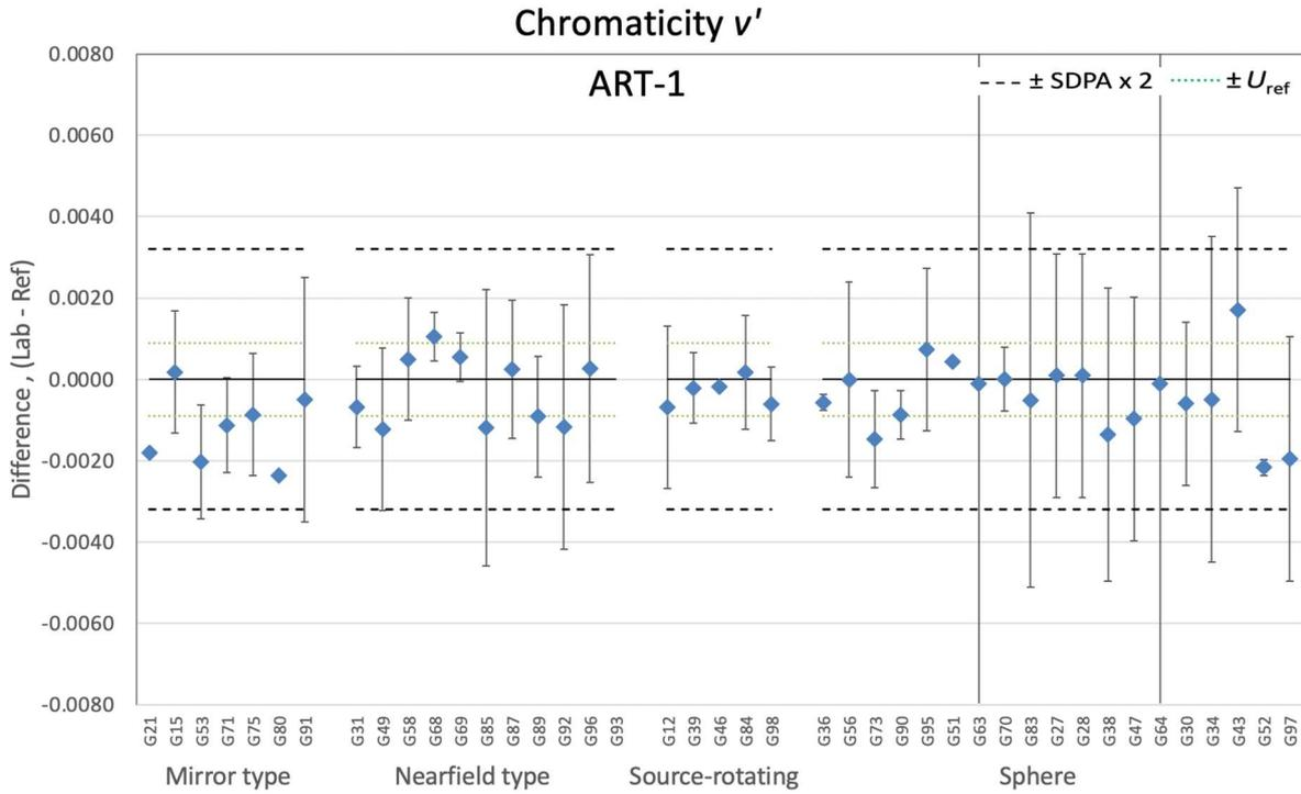
Figure 7-100. Differences of chromaticity  $v'$  for ART-1 by goniophotometer type and sphere
