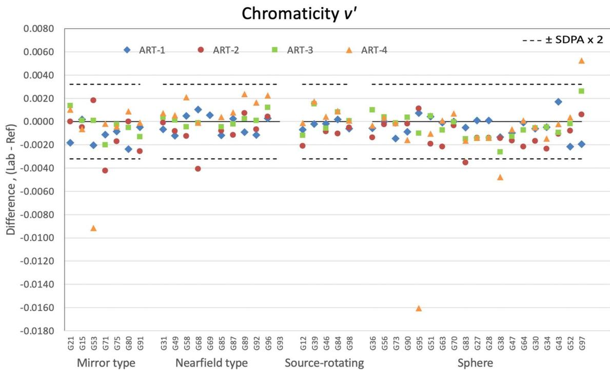
**Figure 7-99. Differences of chromaticity  $v'$  for all artefacts by goniophotometer type and sphere**
