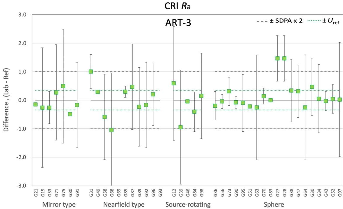
Figure 7-112. Differences of CRI  $R_a$  for ART-3 by goniophotometer type and sphere
