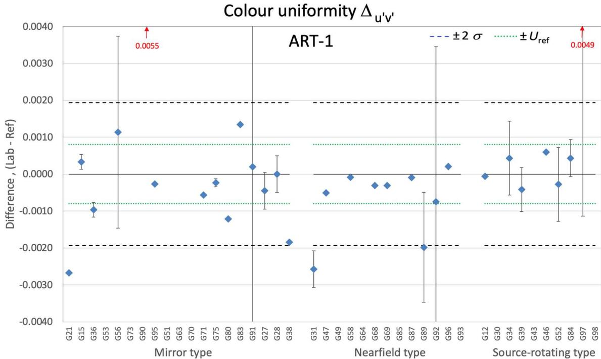
Figure 7-125. Differences of colour uniformity for ART-1 by goniophotometer type
