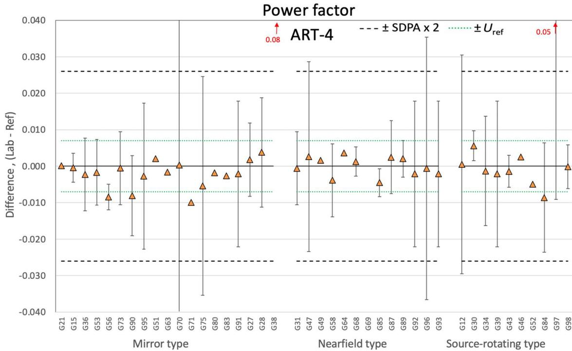
**Figure 7-93. Differences of power factor for ART-4 by goniophotometer type**
