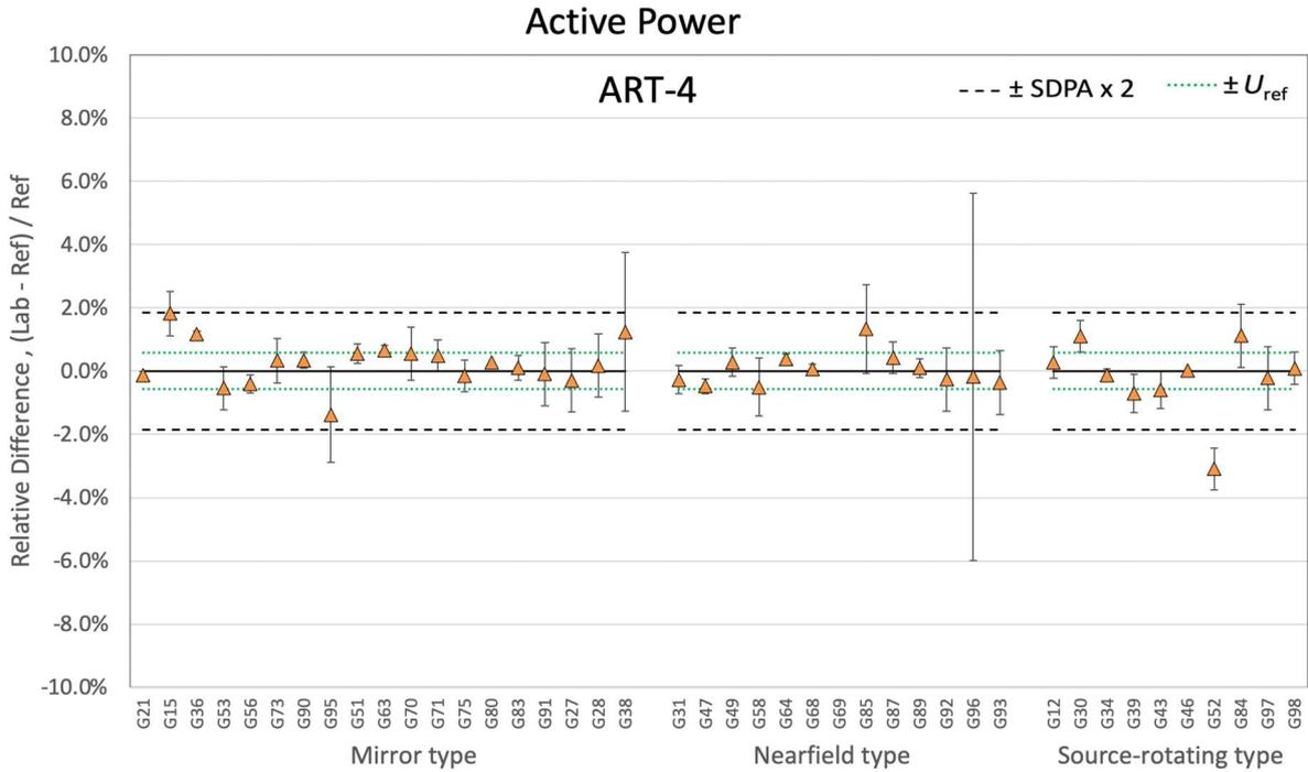
Figure 7-79. Relative differences of active power for ART-4 by goniophotometer type
