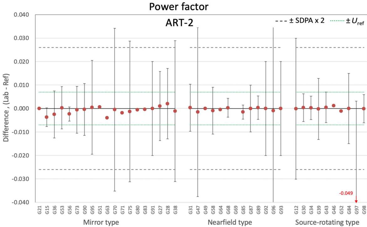
Figure 7-91. Differences of power factor for ART-2 by goniophotometer type
