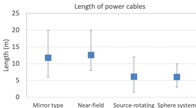
**Figure 7-132. Average length of power cables between power supply and artefacts on the goniophotometer in all participants' labs**
