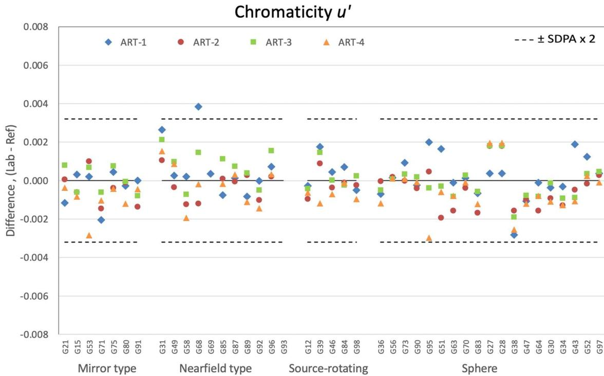
Figure 7-94. Differences of chromaticity  $u'$  for all artefacts by goniophotometer type and sphere
