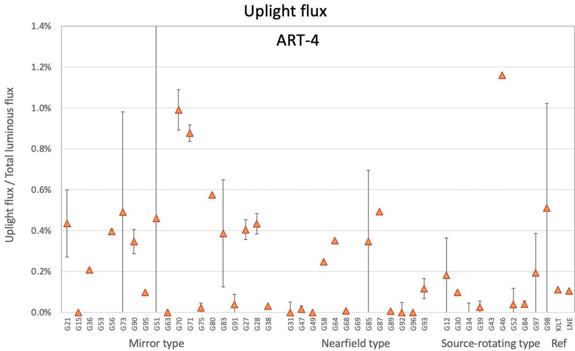
Figure 7-124. Uplight flux relative to total luminous flux for ART-4 by goniophotometer type
