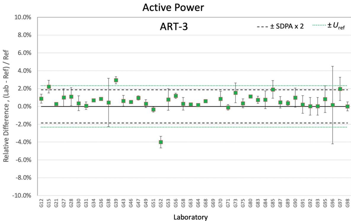
Figure 7-11. Relative differences of active power for ART-3
