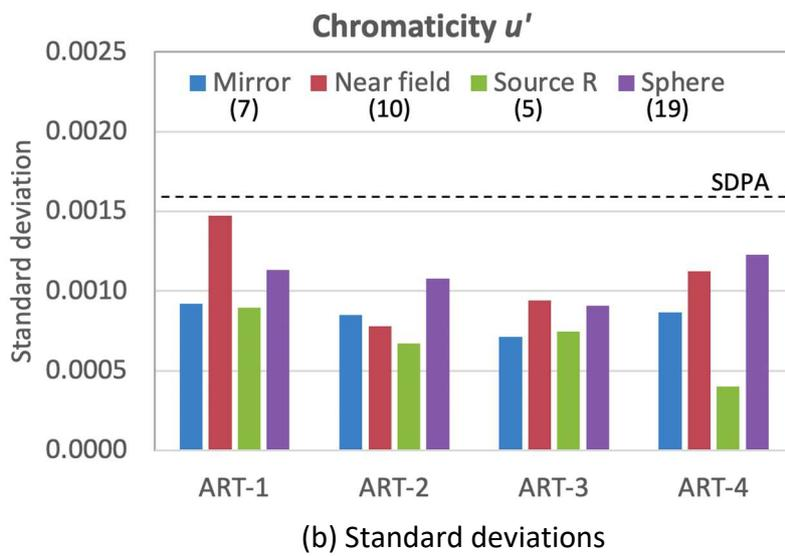
**Figure 7-133. Average deviations from the reference value (a) and the standard deviations (b) of chromaticity  $u'$  results for each instrument type**
