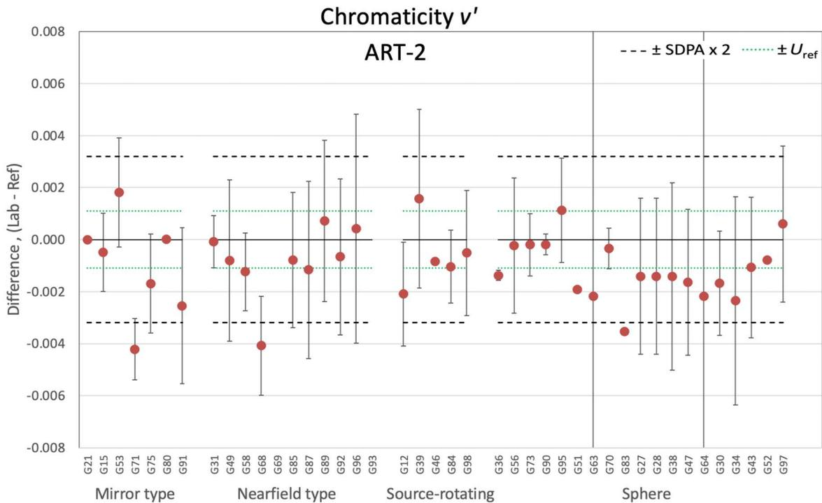
Figure 7-101. Differences of chromaticity  $v'$  for ART-2 by goniophotometer type and sphere
