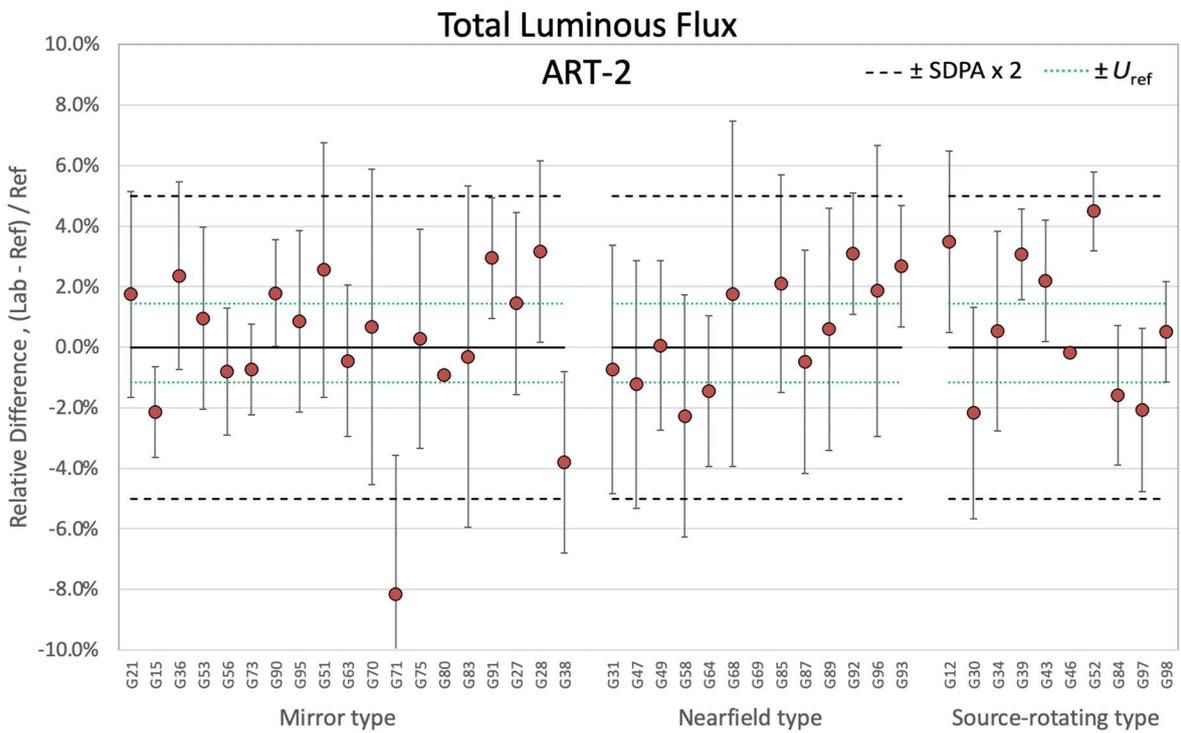
**Figure 7-72. Relative differences of total luminous flux for ART-2 by goniophotometer type**
