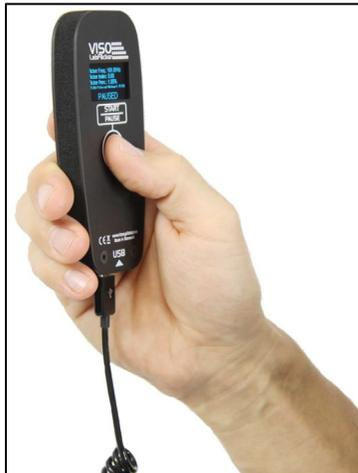
Figure 5. Viso Systems LabFlicker handheld meter.
