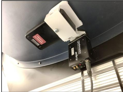
**Figure 3. Handheld meter slid into place on flange, next to the reference meter.**
